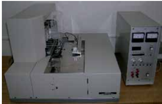
Fig. 1. Device for measurement of fabric surface characteristics
