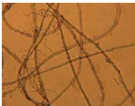
Fig. 5. Fibrillation of lyocell fibre. (Zhang, 2004)
