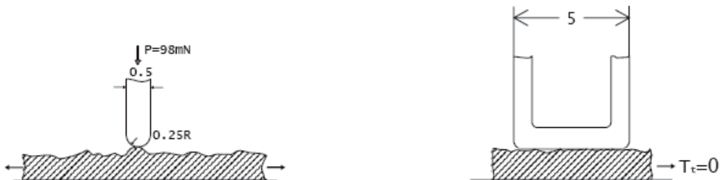
Fig. 2. KES contactor for measuring of surface roughness
