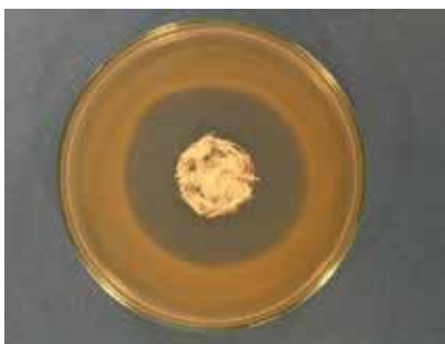
Photo 1. Growth inhibition zone around the S. aureus ; polypropylene fibers containing 2% Ingaguard- method according to SN 195 920
