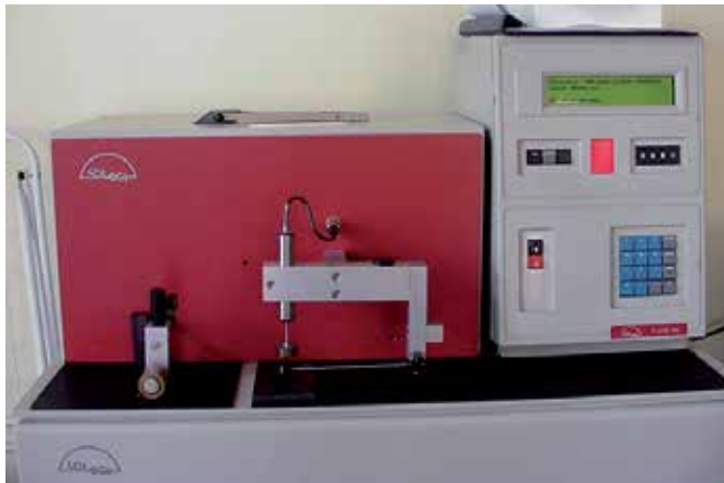
Fig. 5. The step thickness meter SDL M 034/1
