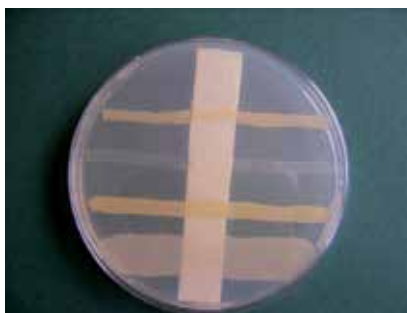
Photo 3. Growth of bacteria respectively from the top: S. aureus , E. coli ; M.flavus , B. licheniformis under polymer with nano-silver - method according to AATCC 147
