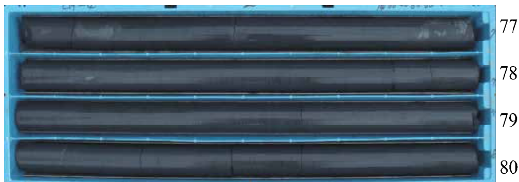
Fig. 2. (b) Rock core photos of borehole CH-04 without fault influence.
