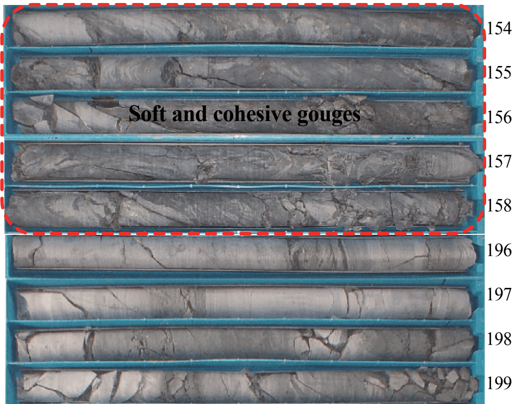
Fig. 2. (a) Rock core photos of borehole HB-95-2 with fault influence.
