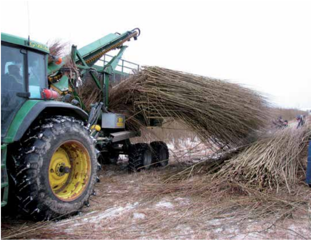
Figure 11. A tractor-pulled whole shoot harvester, unloading willow shoots at the headland (Photo: Nils-Erik Nordh).
