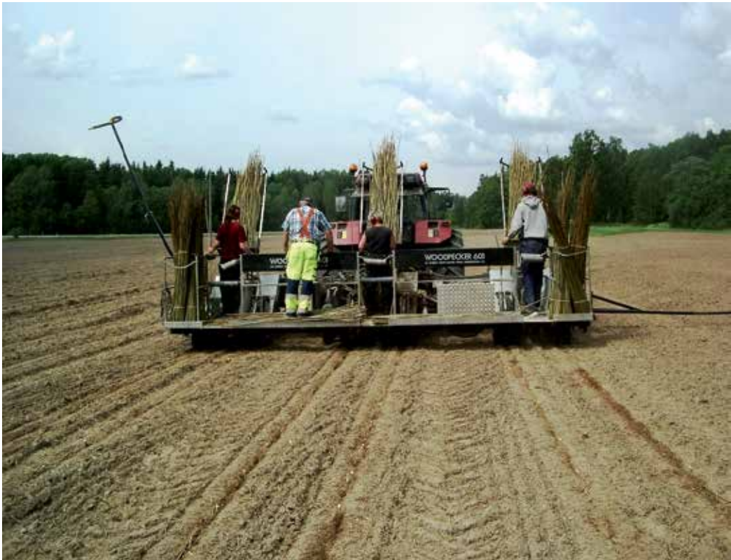
Figure 1. Machine planting of willow by means of a Woodpecker 601, using long rods and planting three double rows at a time (Photo: Nils-Erik Nordh).
