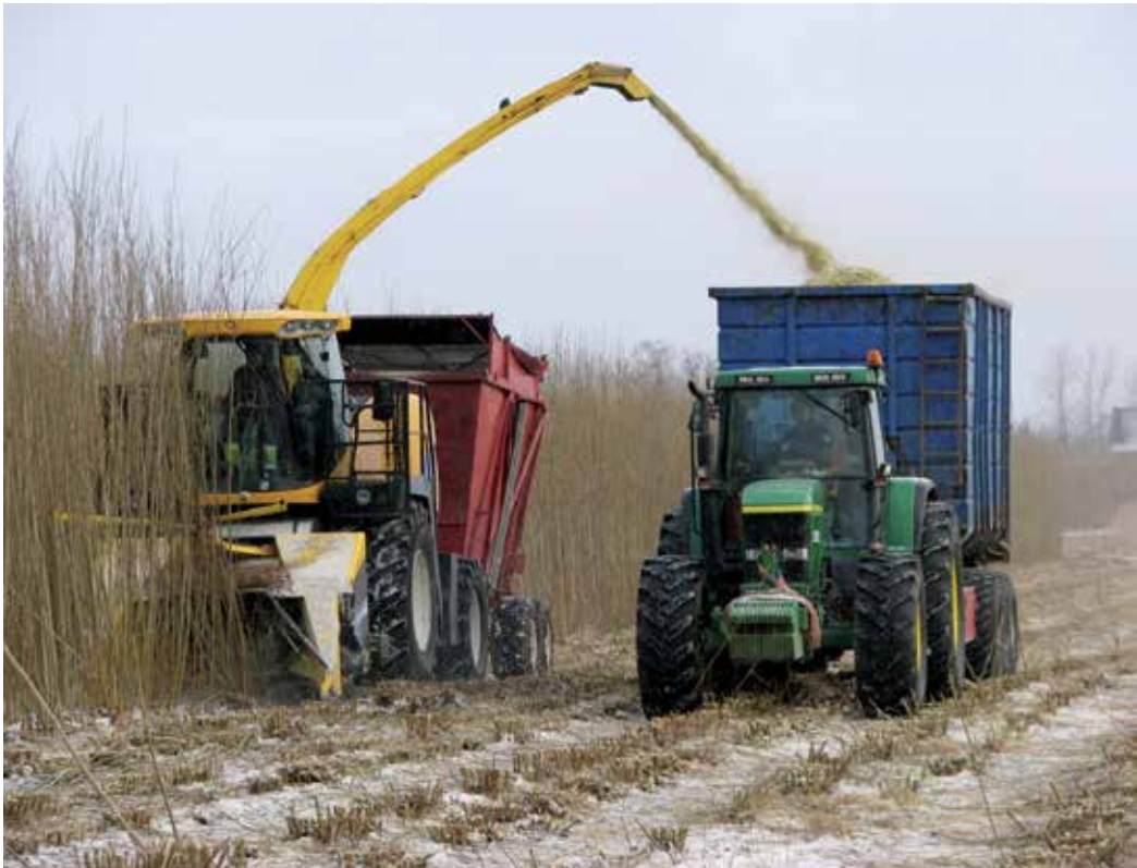
Figure 9. Willow harvest by means of a self-propelled chipper which blows the willow chips in an adjacent container (Photo: Nils-Erik Nordh).
