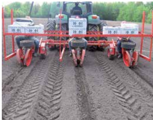
Figure 1. Willow planting machine operating on 3 rows simultaneously
