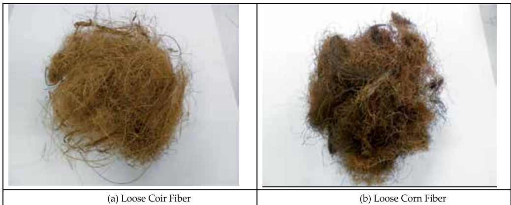
Figure 1. Loose forms (a) Coir Fiber (b) Corn Fiber
