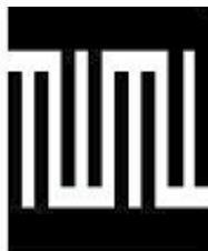
Figure 21. Structure of delaying line converters
