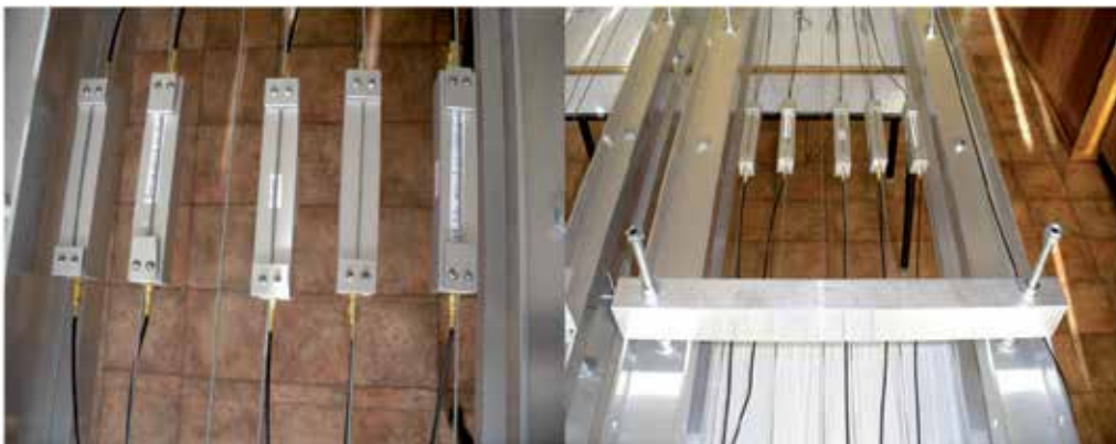
Figure 44. SAW-comprising vibration sensors attached to steel ropes
