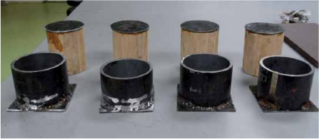
Figure 4. Steel molds and wooden punches were used to fabricate the samples.
