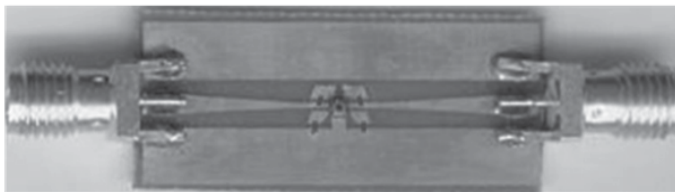
Figure 15. Tunable BAW-SMR filter and passive elements mounted on FR4 PCB.
