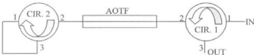
Figure 10. Double pass configuration to increase the maximum attenuation of the notch filter.
