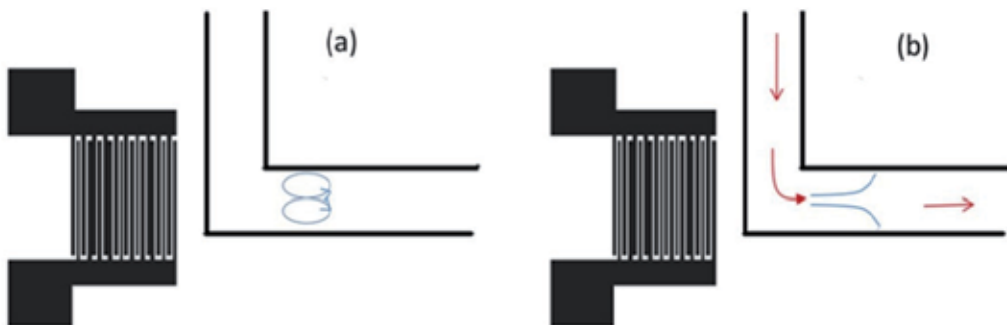
Figure 18. Principle of SAW-based micropumps with a channel. When the vortex is smaller than the channel width, the back flow occurs, suitable for in-channel mixing (a). When the vortex is larger than the channel width, a unidirectional flow is formed (b).
