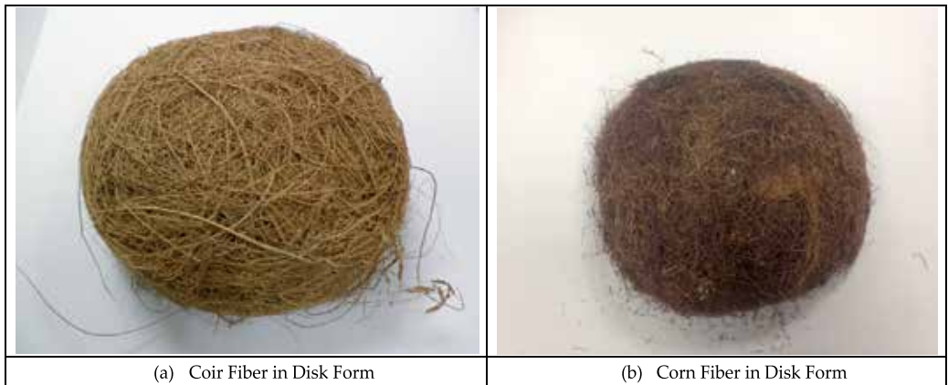
Figure 2. Fibers in disk forms (a) Coir fiber (b) Corn fiber
