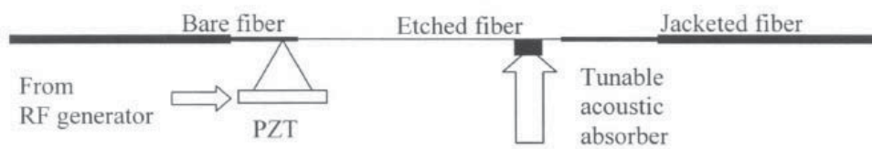
Figure 8. Setup to study the bandwidth variation using the AO interaction inside fiber.
