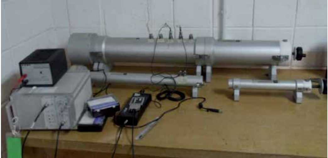
Figure 5. Measurement apparatuses consisting of impedance tubes, noise generator and 01dB analyzer.
