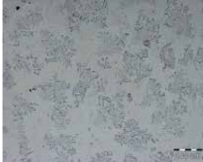
Figure 6. Microstructure of alloy Ni 50.6 -Ti (at. %), EBM
