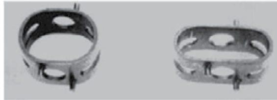
Figure 2. Spinal vertebrae spacer (Duerig, Melton et al. 1990)
