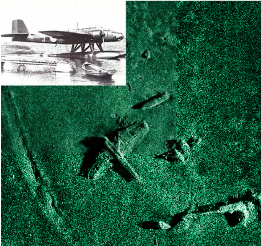
Fig. 18. SAS image of a German WWII Heinkel He 115 seaplane lying on the seafloor. Courtesy of the Royal Norwegian Navy. Photograph is from wikipedia.
