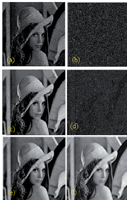
Fig. 17. A comparison of three despecklisation methods acting in the wavelets domain; (a) noisy image (PSNR=21.4 dB), (b) speckle noise distributed following a Rayleigh law with unitary mean, (c) result obtained with the method based on 2D DT CWT (PSNR=31.4 dB), (d) 2D DT CWT method's noise, (e) result obtained with the method based on HWT (PSNR=32.5 dB), (f) result obtained with the method in [Argenti et al., 2006] (PSNR=31.1 dB).
