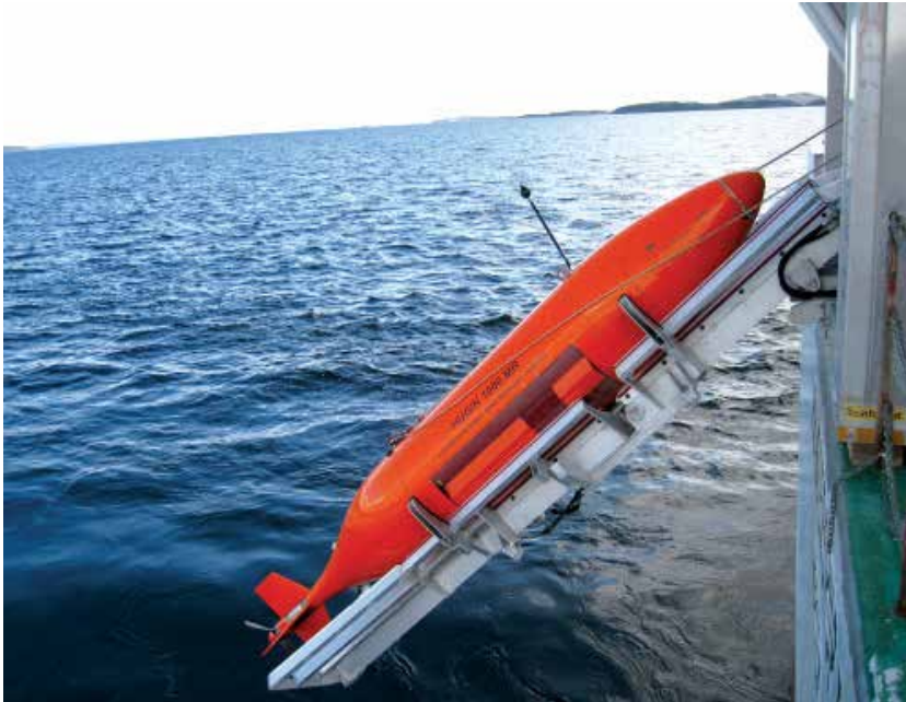
Fig. 15. The HISAS 1030 interferometric SAS on the HUGIN autonomous underwater vehicle. The picture was taken just before launch during a scientific mission on board the research vessel H U Sverdrup II in Norwegian waters in April 2010.
