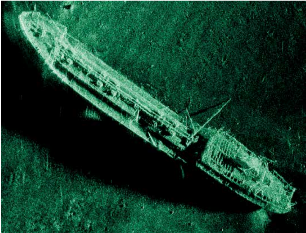
Fig. 16. SAS image of the wreck of the Norwegian tanker Holmengraa that was sunk during WWII in 1944. Courtesy of Kongsberg Maritime.
