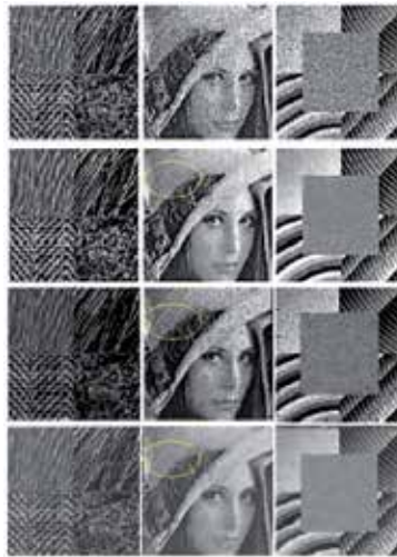
Fig. 16. A comparison of the visual aspect of the results of three despecklisation methods; From up to bottom: noisy sub-images, results obtained applying the method in [Walessa&Datcu, 2000], results obtained applying the method in [Ifremer, 2010] and results obtained applying the method based on the HWT.
