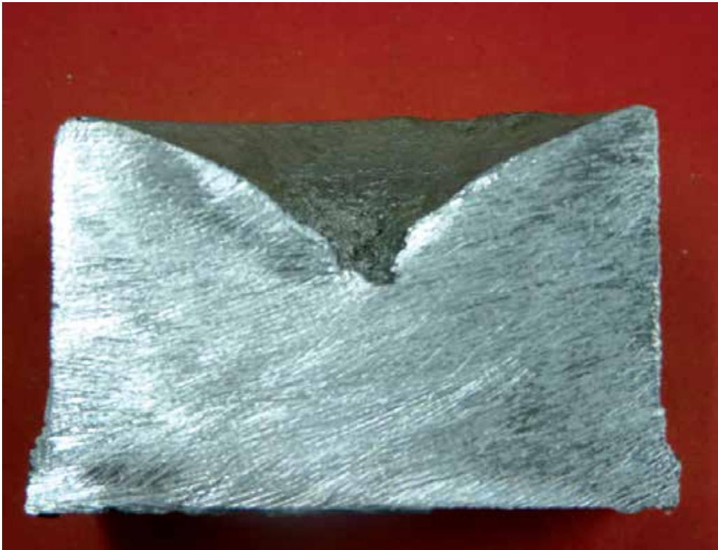
Fig. 7. Typical appearance of volumetric shrinkage defect in an aluminium section
