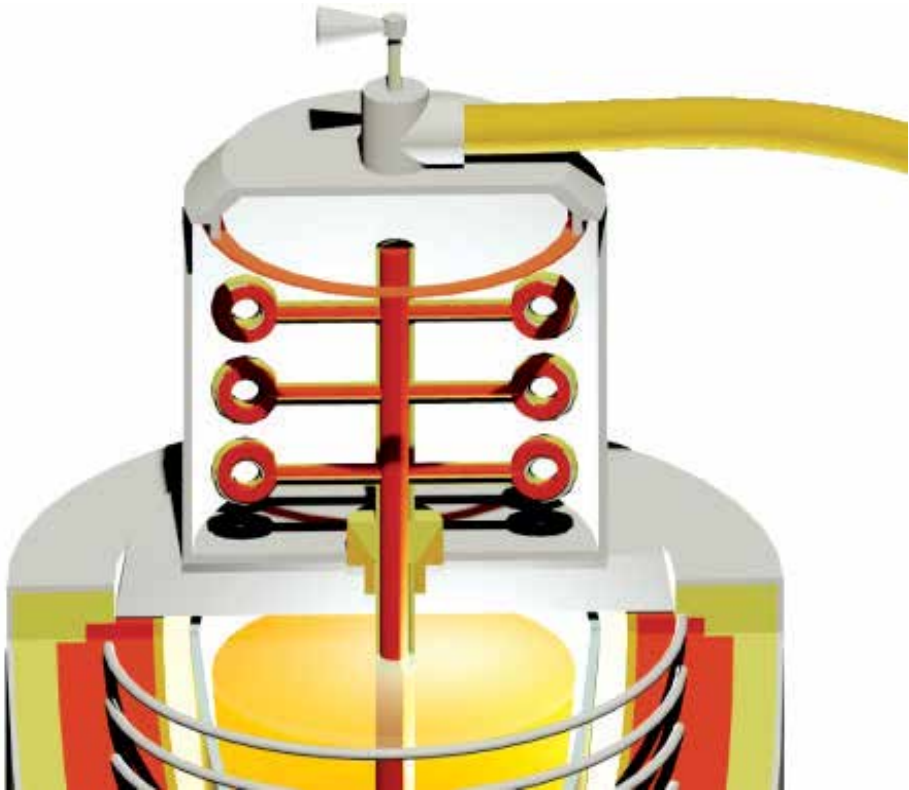
Fig. 4. The vacuum is maintained until the cavity is completely filled. Vacuum pressure is released causing un-solidified melt to flow back into the furnace
