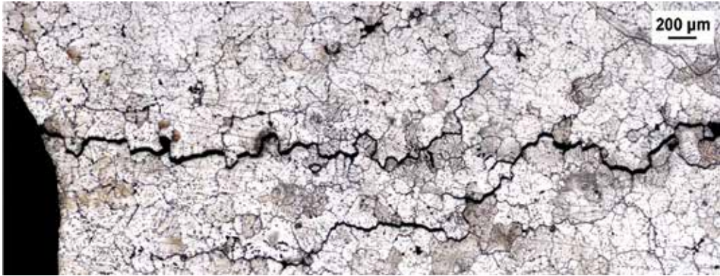
Fig. 14. Fracture path developed by coalescence of shrinkage porosity due to quenching of liquid phase
