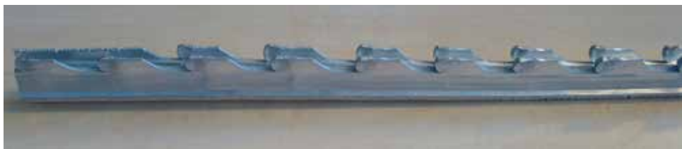
Fig. 1. Extreme case of hot tearing in AA7075 aluminum alloy [3]
