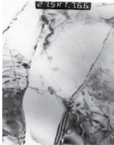
Fig. 8. TEM micrograph of Al 6013/SiC interface showing dislocation generations
