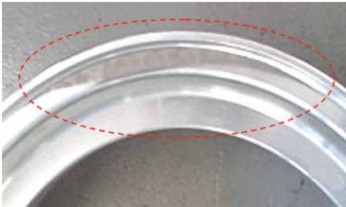
Fig. 8. Wheel distortion after post-cast cooling in water at a temperature of 30^{\circ}\text{C}
