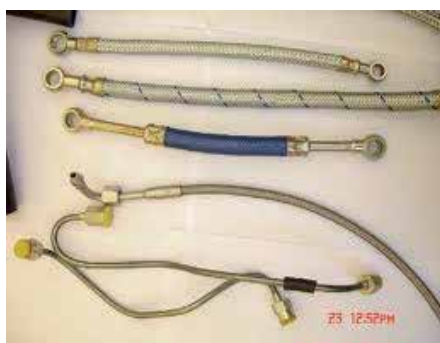
Fig. 25. Alodine coated Fuel Injection Fuel Lines
