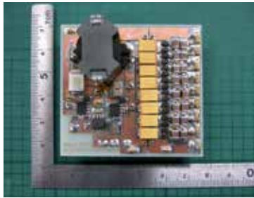
Figure 21. Photograph of a 10-W prototype of the double-switch series-resonant equalizer using a voltage multiplier for 8 cells connected in series.
