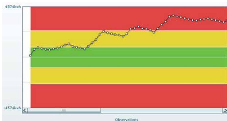
Fig. 10. CuSum of the hydraulic press energy consumption
