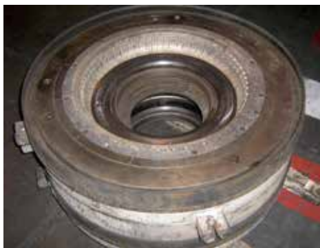
Fig. 5. a) Monoblock tyre vulcanization mould system b) 1/8 of tread ring segment.
