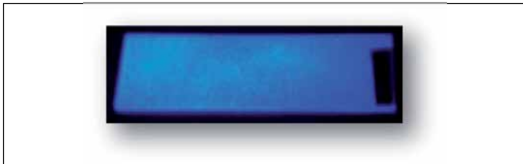
Fig. 27. Picture of a BAM:Eu 2+ film under UV excitation.
