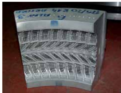
Fig. 5. a) Monoblock tyre vulcanization mould system b) 1/8 of tread ring segment.
