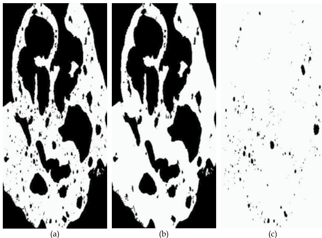
Fig. 4. Reconstructed slice showing the total porosity after binarisation (a), open porosity after region growing (b) and closed porosity (c).
