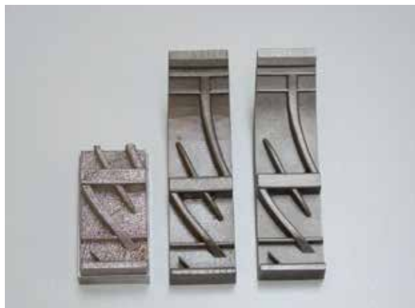
Fig. 6. The one-pitch-segments made by SLM, SLS and DMLS technology.
