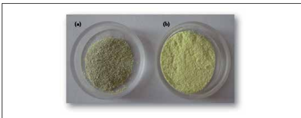
Fig. 3. Picture of as-synthesized YAG:Ce powder before(a) and after(b) post-calcination at 1000°C for 2 hours.
