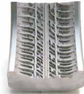
Fig. 4. Tread ring segment made by engraving on CNC.
