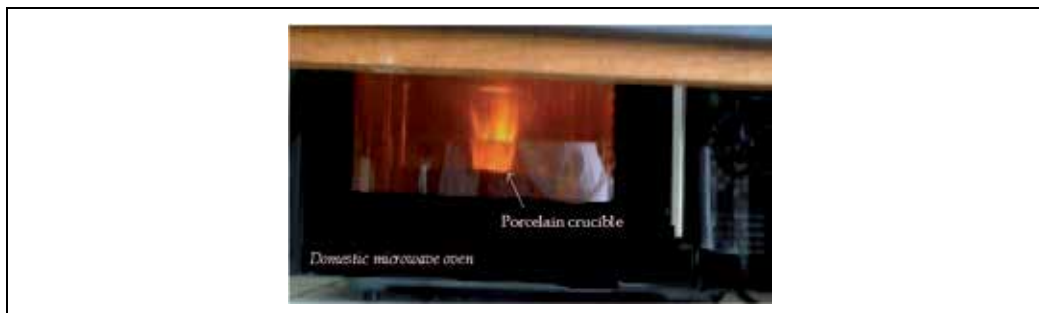
Fig. 1. Picture of a porcelain crucible containing nitrates/urea solution, ignited after few minutes of microwave irradiation.
