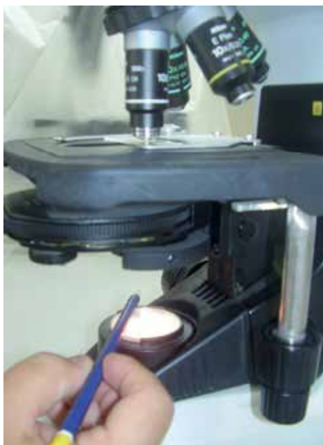
Fig. 6. An opaque object – a pencil– is placed between the lamp and the sample to simulate the phase contrast technique.
