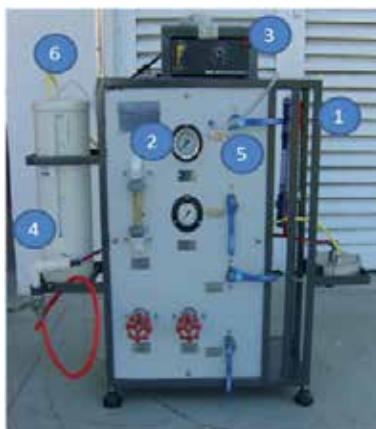
Fig. 2. Frontal view of the MF/UF module (Operation manual – MF/UF module): (1) polymeric membranes; (2) pressure gauges; (3) speed controller; (4) feed tank; (5) valve used to collect the permeate; (6) tubing through which the concentrate returned to the feed tank.
