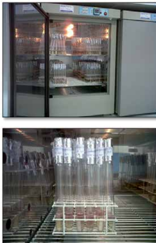
Fig. 7 and 8. Performance of the sterility test by direct incubation in samples submitted to ethylene oxide.
