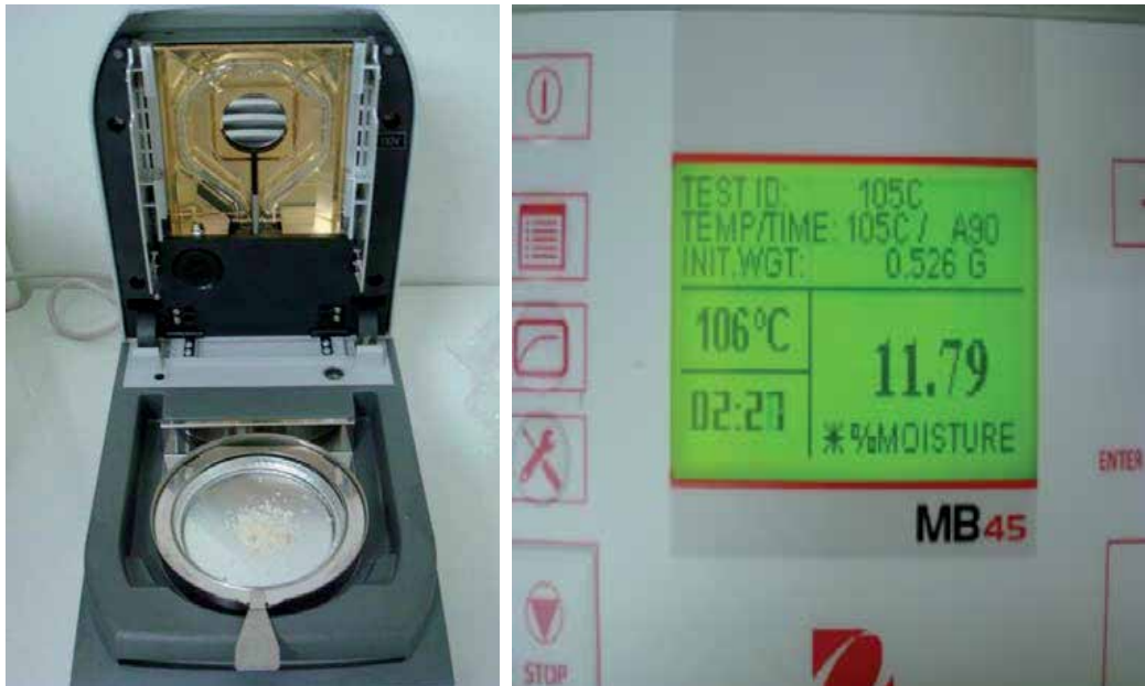
Illustrations 12,13. Residual Moisture Analyzer: Ohaus® equipment belonging to the Tissue Bank of Hospital das Clínicas – Universidade de São Paulo.
