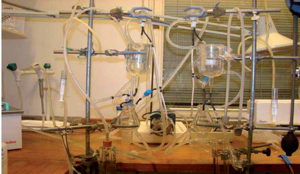
Fig. 2. Photograph of the in vitro perfusion apparatus
