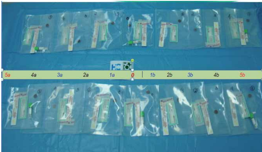
Fig. 6. Samples of packaging positioned from 0 to 5 for EtO penetration analysis.
