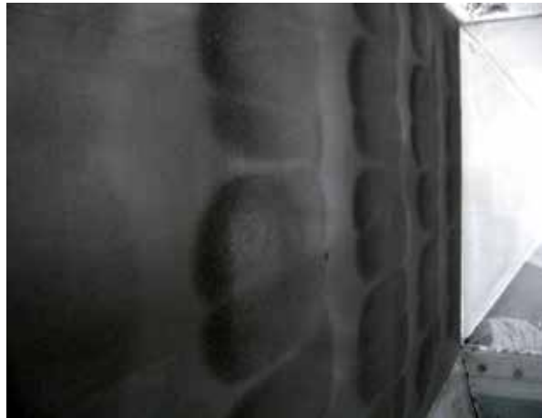
Fig. 23. Pattern of collected fly ash on CE electrodes for RDE-3 electrode.
