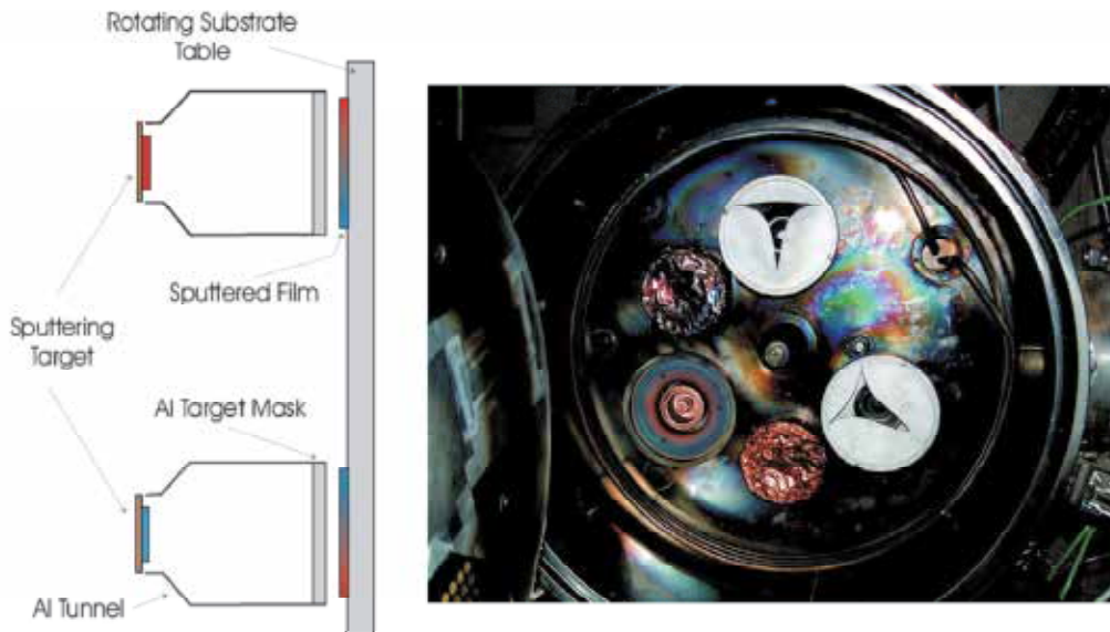
Fig. 5. Schematic side view (left) and actual (right) front-view image of the sputtering machine set-up with linear-in (at 4:00) and linear-out (at 12:00) masks placed in front of each target (color on-line).
