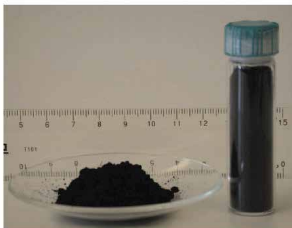
Fig. 3. Example of the bulk quantity of graphene product. The image consists of approximately 2 g of sample (Choucair, M. et al., 2009).
