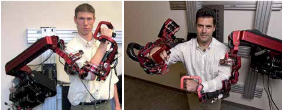
Fig. 17. Rosen and et al.'s 7DOF Manipulator EXO-7 (Perry, 2007; Yu & Rosen, 2010)
