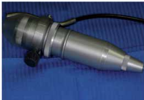
Fig. 20. Specially designed Nd: YAG laser tip for intraoral metal welding. (Courtesy of Prof. Carlo Forniani)
