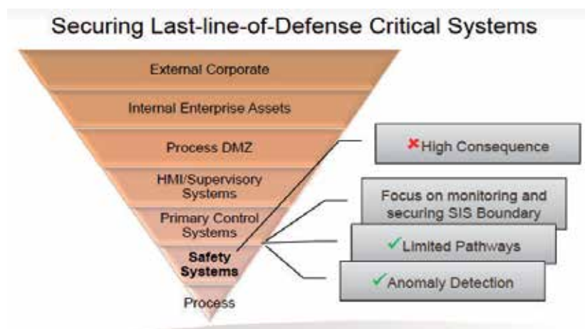
Fig. 19. Position and mechanisms enabling Last-line-of-Defense.
