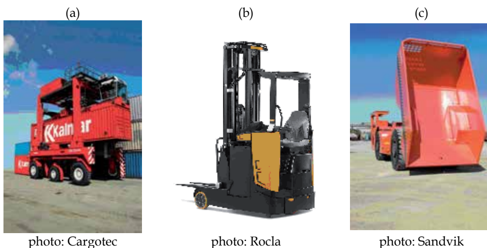
Fig. 1. Examples of mobile working machines: a) straddle carrier, b) forklift truck and c) mine underground truck. (Minav, 2011d)
