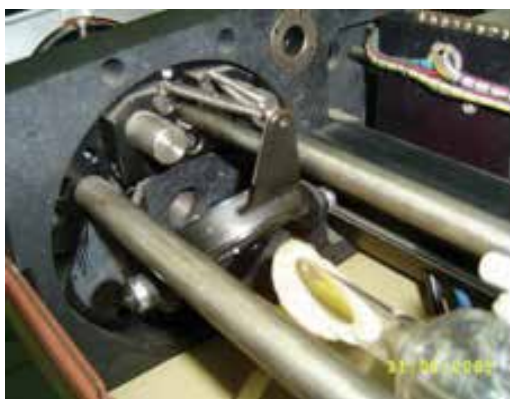
Fig. 6. Diffraction grating-drive mechanism.
