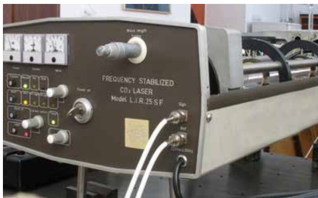
Fig. 5. Homebuilt frequency stabilized CO 2 laser model LIR-25 SF.
