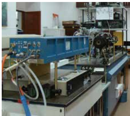
Fig. 10. Coherent GEM SELECT 50™ CO 2 laser in the experimental setup.
