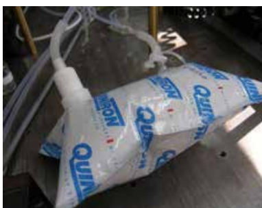
Fig. 20. Aluminum-coated plastic bag with sample gas.
