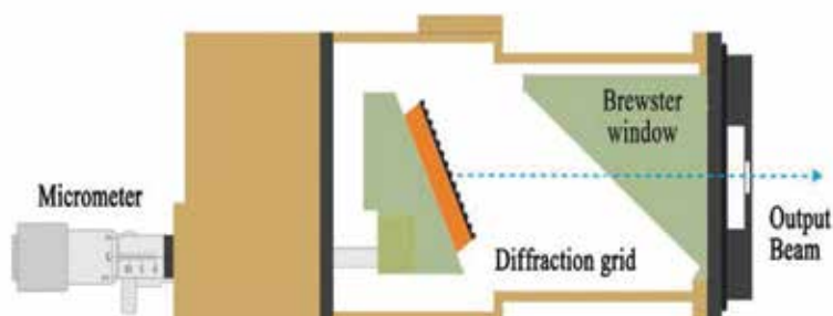
Fig. 1. Schematics of the MTL3-GT TEA laser from Edinburgh Instruments [6]
