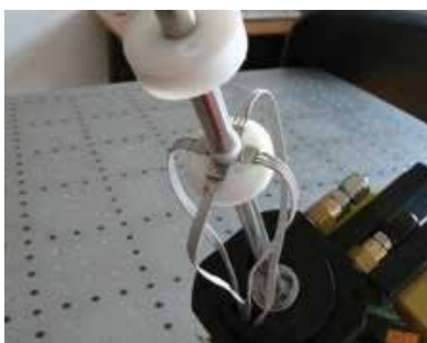
Fig. 14. Teflon rings used to mount the microphones flush with the tube wall.
