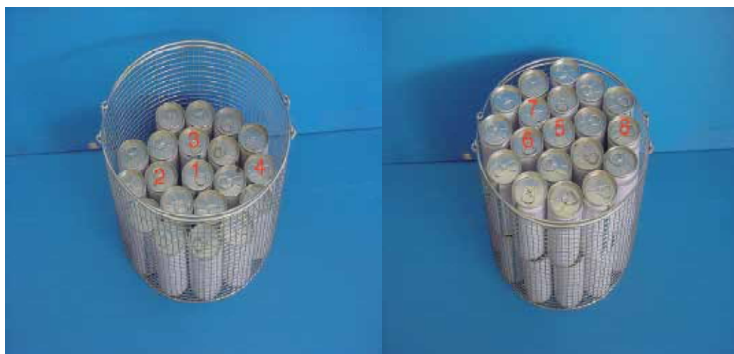
Fig. 7. Location of cans which connected to thermocouples in the basket
