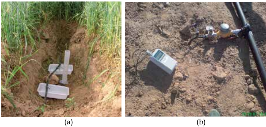
Fig. 10. Field evaluation of SDI units: (a) sample with unearthed emitters and (b) manometer and flow-meter for recording head pressure and inlet flow in laterals.
