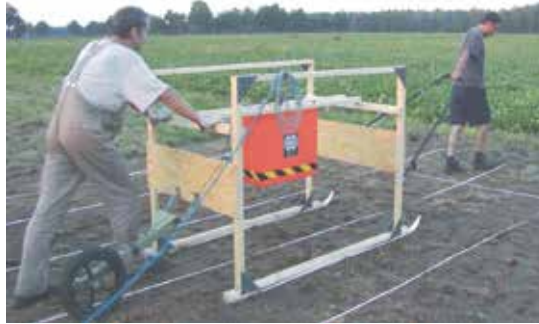
Fig. 12. Experimental setup to determine the coefficient of reflection. A 1-GHz horn antenna is mounted on a sledge 0.5 m above the ground.
