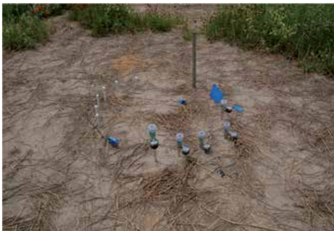
Fig. 5. Use of tensiometers to determine soil matric potential at different soil depths.
