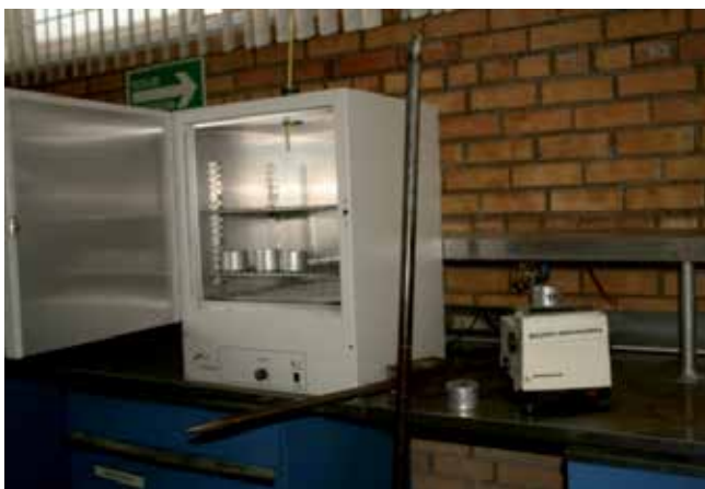
Fig. 2. Equipment used by the gravimetric technique for measuring soil water content.
