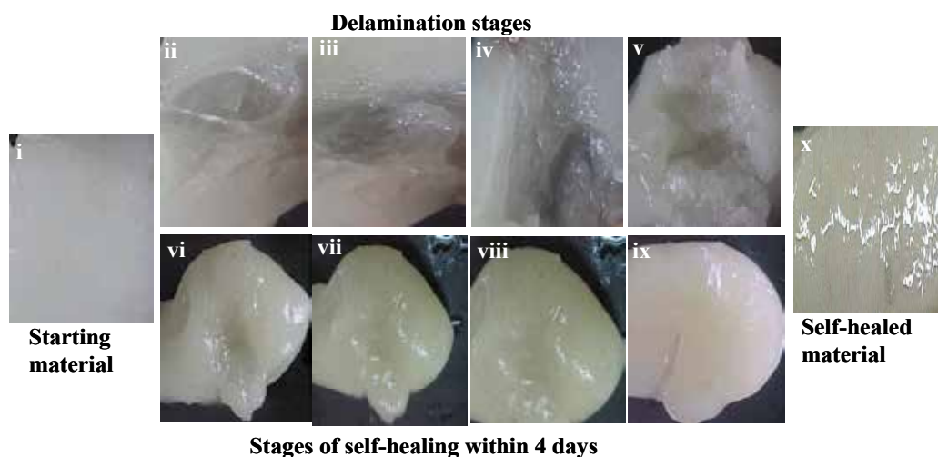
Fig. 5. Self-healing pattern of delamination damages of STLM.
