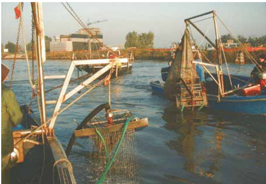
Fig. 9. Hydraulic clam dredge "idrorasca"
