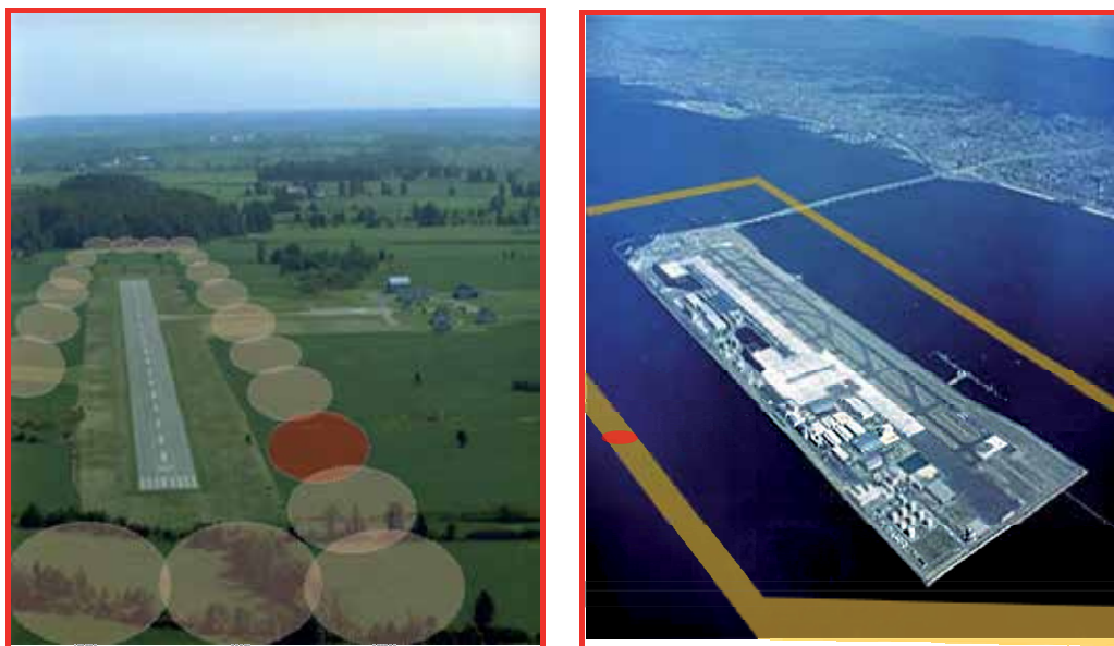
Fig. 9-10. The SFCO -sensor based Early Warning Security System can secure the runway and specific underwater perimeter with the invisible and totally passive security net, and can detect over the ground and underground, as well as underwater moving intruders.
