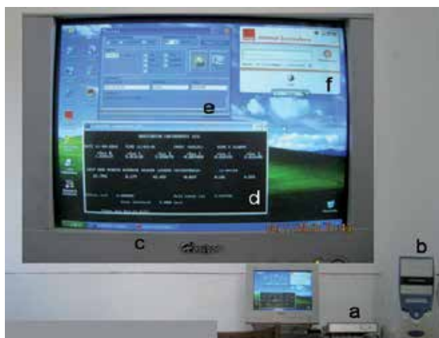
Fig. 7. Monitoring system of the geomagnetic components ( B_x , B_y and B_z ) and real time data transfer : acquisition module MAG-03DAM (a); computer (b) for data storage; monitor (c) for real time geomagnetic data display (d); data transfer program (e) ; wireless connection (f)
