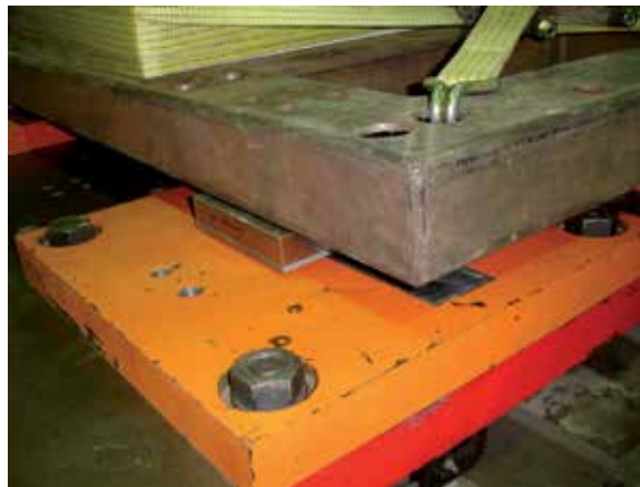
Fig. 20(a). Assembly of direction optimized friction pendulum system
