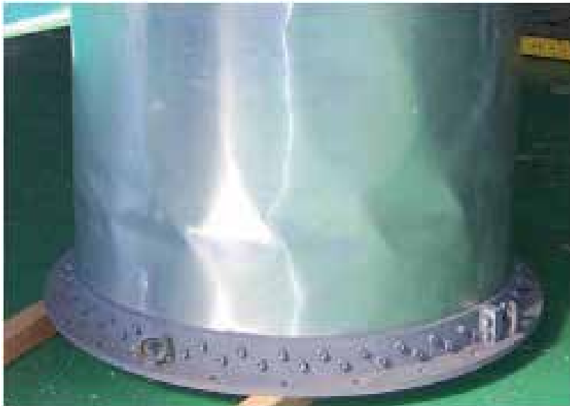
Fig. 2. Typical mode of diamond buckling.
