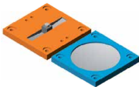
Fig. 11(a). Open-up view of first type direction optimized-friction pendulum system
