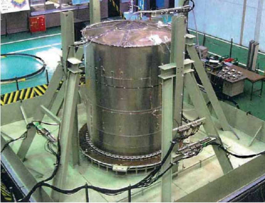
Fig. 19. Large test tank of 1/5 reduced-scale cylindrical liquid storage tank. (Ito et al., 2003)
