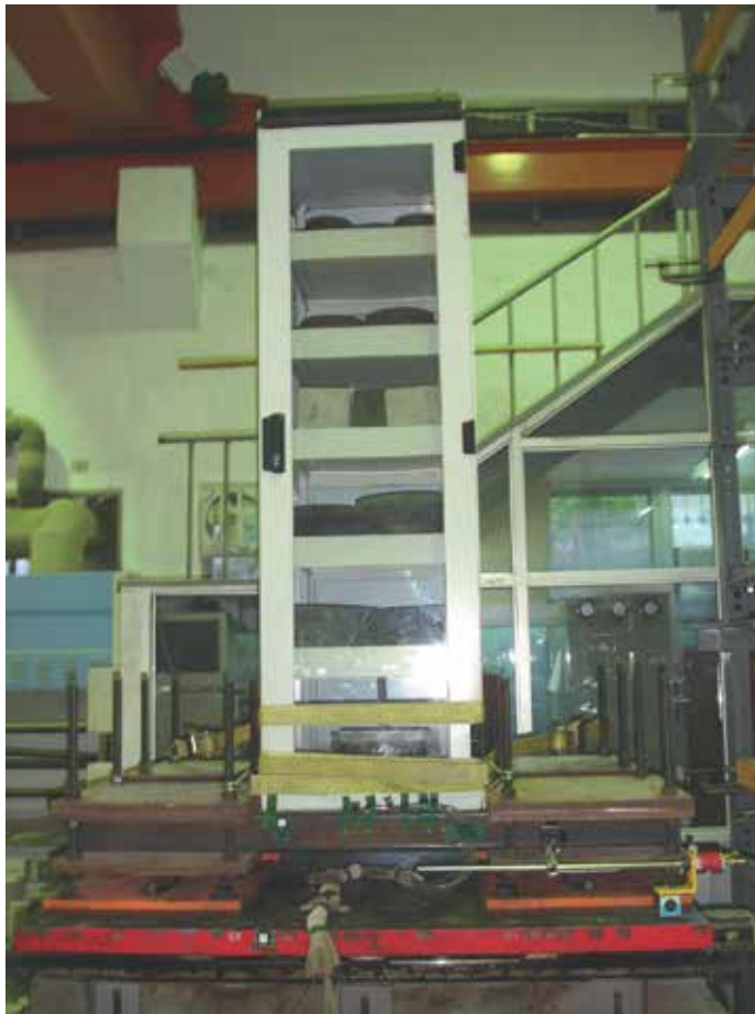
Fig. 31. Critical equipment isolated with DO-FPS isolators
