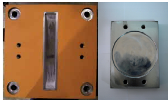
Fig. 20(b). An open-up view of the DO-FPS isolator with trench and concave surface
