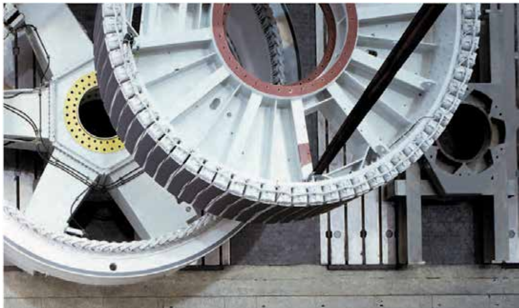
Fig. 5. Rotor and stator of Enercon E-70 wind turbine (Photo: Enercon).
