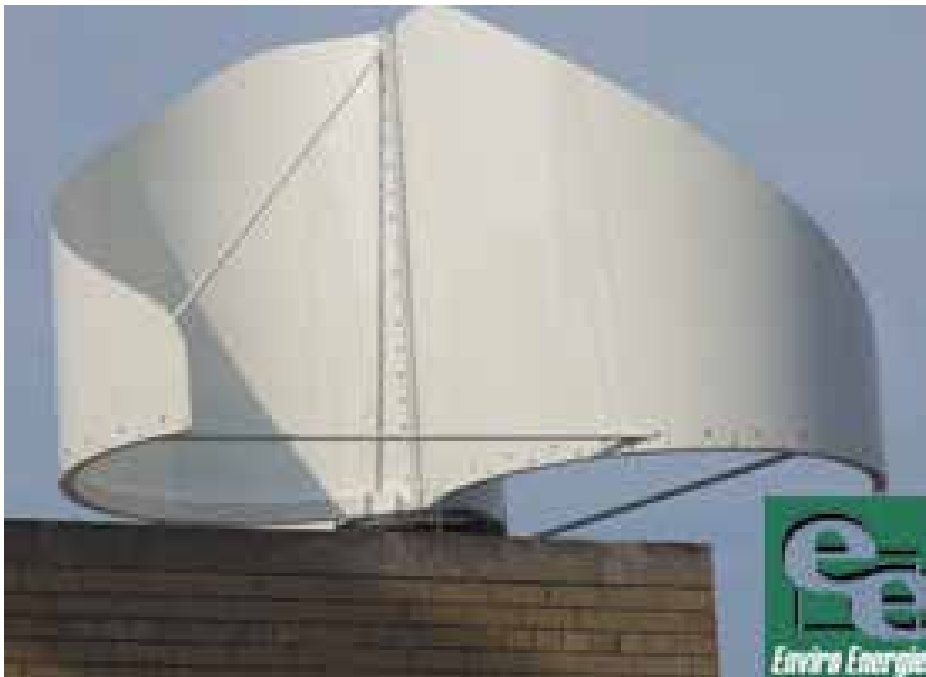
Fig. 2. VAWT made by Enviro-Energies and installed on the company's roof
