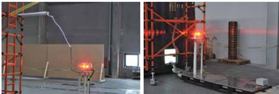
Fig. 5. A test of aircraft warning light, conducted using both impulse voltages and impulse currents, BTI Light systems A/S and Testinglab Denmark ApS.
