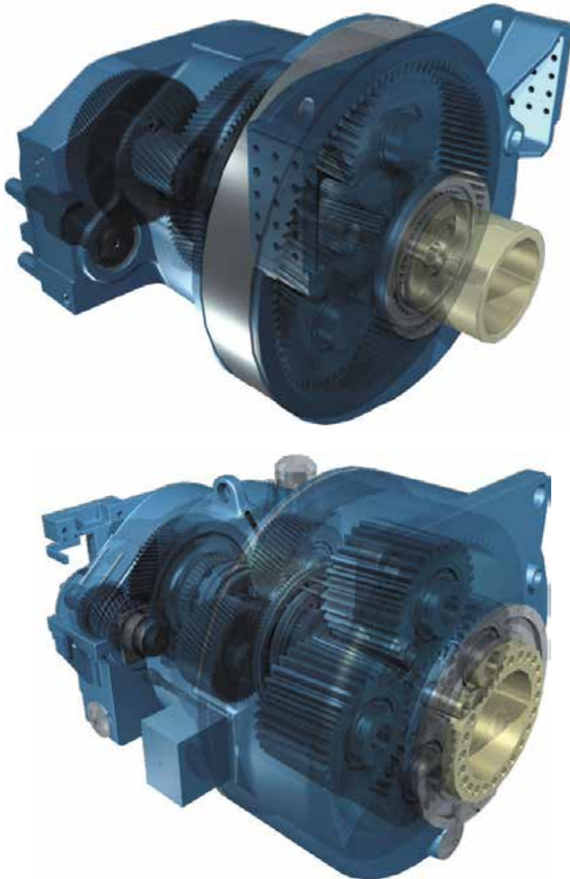
Fig. 3. GE 1P 2.3 one-stage planetary and two-stage parallel shaft (top) and 2P 2.9 two-stage planetary and one-stage parallel shaft (bottom) wind turbine gearboxes (Image: GE).
