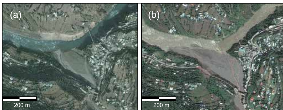
Fig. 10. (a) Satellite image of the junction of the Karli River with the Jhelum River before and after the breaching of Hattian dam (Google earth)
