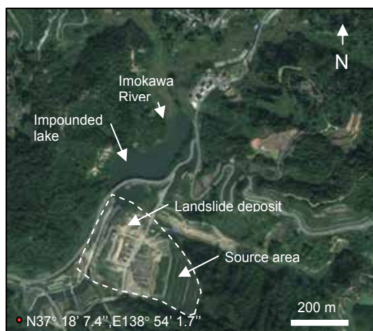
Fig. 3. Higashi Takezawa landslide dam and the dammed lake (Satellite imagery from Google Map)
