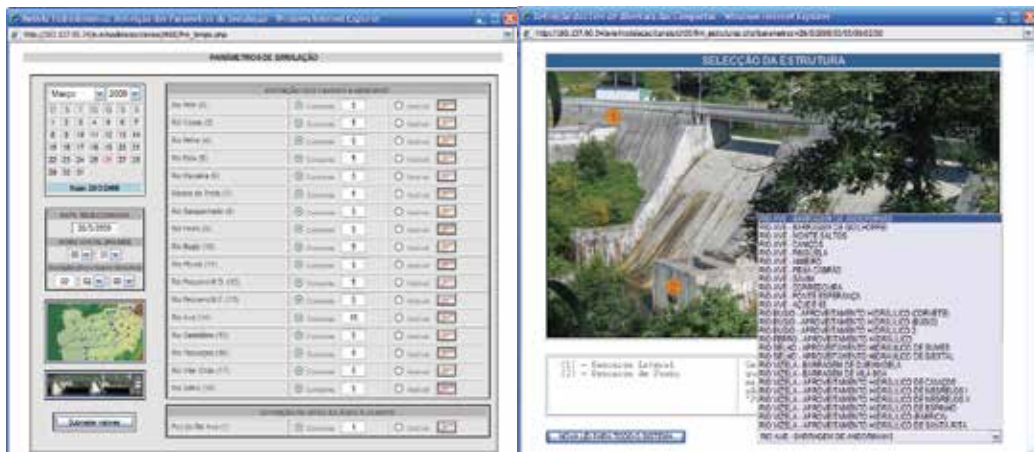
Fig. 11. Main form for definition of new simulations data (left) and interface to define data time series related to hydraulic structures (right)
