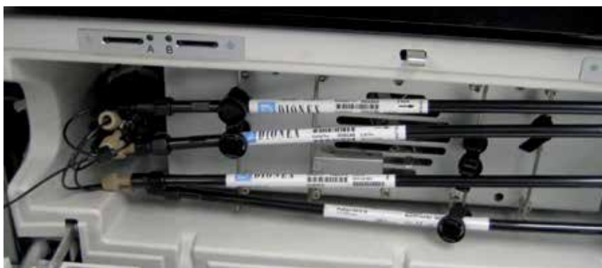
Fig. 13. HPLC column compartment equipped with a 6-port column switching valve, for screening of up to six different columns for pH-IEC without the need to change buffers or columns.
