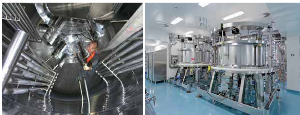
Fig. 1. Left side: photograph of a 15m 3 state of the art sterile containment for high cell density fermentations. LONZA has built and operates such high performance equipment up to the 75m 3 for a range of organisms including methylotrophic yeasts such as Pichia pastoris . The flow breakers are designed as cooling elements needed to remove metabolic heat. The stirrers are concave Rushton impellers which, in combination with specially designed dip pipes (not shown), allow optimal mixing. In most cases the stirrer configuration is completed by the use of a top radially downward pumping marine impeller. Right: Two chromatography columns for the purification of injectable therapeutic proteins with a diameter of 2 meters to demonstrate size and complexity of down stream processing (Copyright@Lonza).
