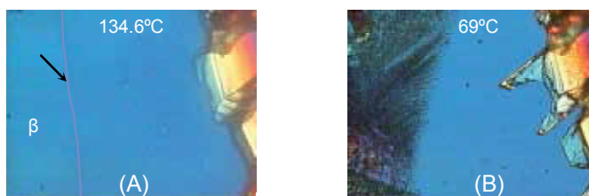
Fig. 8. Micrographs registered during cooling of pindolol from melt. (A): As crystallization is initiated, the \beta phase is separated out; the boundary of \beta is indicated in the picture by an arrow as eye guide. (B): crystallization of both domains.
