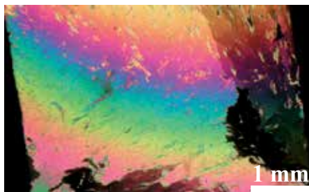
Fig. 5. Image taken under the optical microscope of TPB grown from the melted compound on a functionalized quartz substrate. The image was taken with crossed polarizer and analyzer for a generic orientation of the crystal, so that both interference and birefringence (but mainly birefringence) contribute to give the observed fringes in regions of different thickness.
