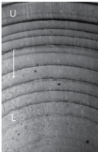
Fig. 4. Micromorphology of a vertical, side (111) surface. U, L-upper and lower parts of a crystal. Arrow indicates direction of gravitational field. Growth temperature: 25 °C. Field of view: 2.7 mm x 4 mm.
