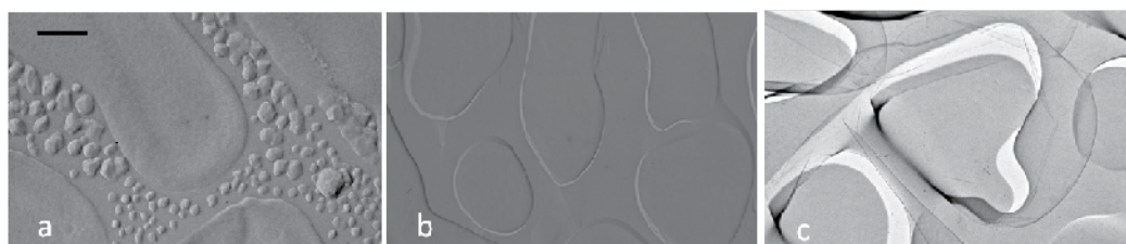
Fig. 5. TEM images of the ice surface formed from trehalose solution (35 wt%) fractured at temperatures (a) approximately 90 K, (b) approximately 180 K, and (c) approximately 250 K. Scale bar: 500 nm. (Reprinted from Uchida et al., 2007, with permission from Elsevier with slight arrangement.)
