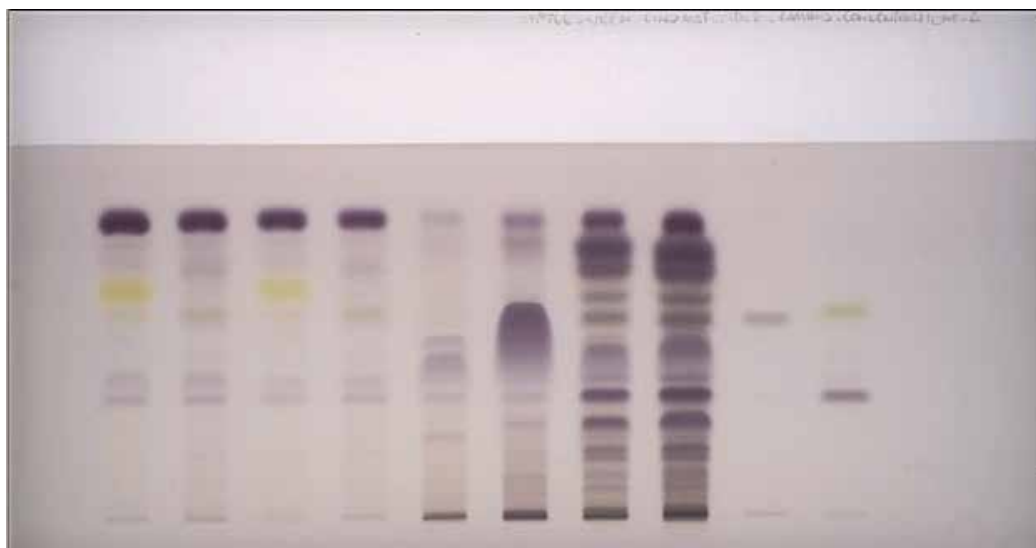
Fig. 4. HPTLC analysis of selected neem cakes. Tracks 1-6 fingerprints of six marketed neem cakes; tracks 7-8 neem cake of track 6 reextracted with ethylacetate and defatted in two concentrations; track 9 nimbin; track 10 salannin.
