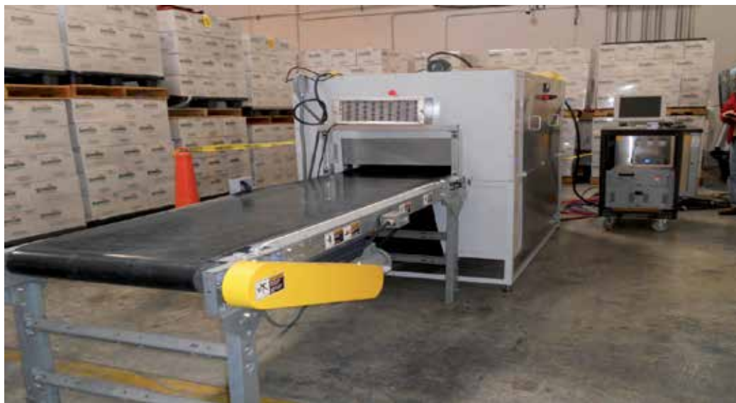
Fig. 4. RF system for batch processing (13.15 MHz, 10 kW). Designed by UC Davis & RF Biocidics Inc.
