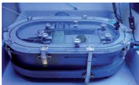
Fig. 4. Measurement of oxygen evolution. A coral colony is held in an enclosure equipped with an oxygen sensor, a paddle wheel, and a water jacket for temperature control. Light is supplied from the top.
