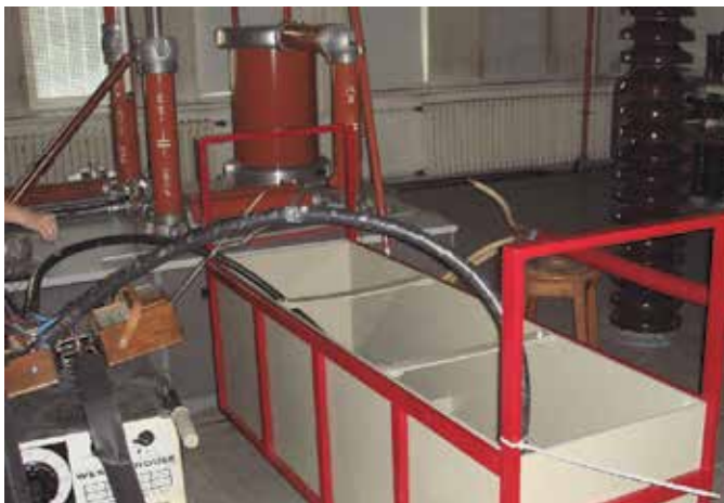
Fig. 15. Experimental set-up for 0.6/1 kV cable.
