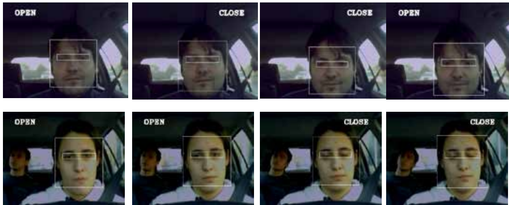
Fig. 3. Output of the driver alertness monitoring system with two video sequences.
