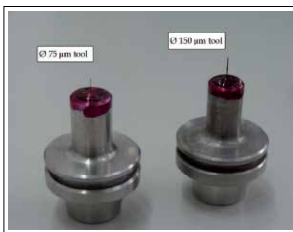
Fig. 9. Tools ready for manufacturing. The left tool has a diameter of 75 \mu\text{m} and the right tool a diameter of 150 \mu\text{m} , both with Lacomit layer.
