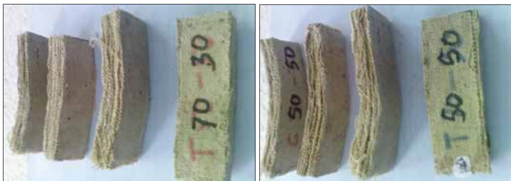
(a) bending specimens biosized 70:30
