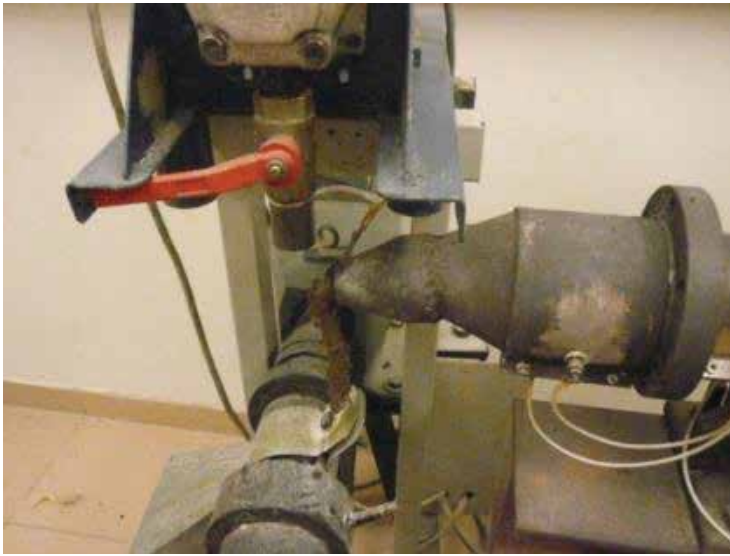
Fig. 4. The hot extrudates coming out of the extruder
