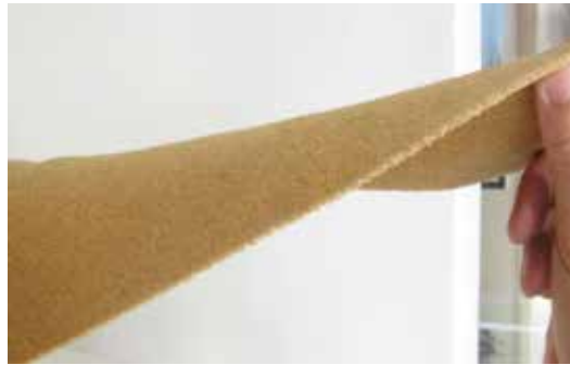
Fig. 18. Flexible sheet of PVB/wood flour (60/40) composite
