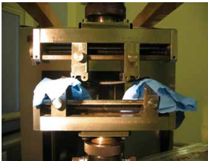
Fig. 10. Experimental setup for 4PBT specimens
