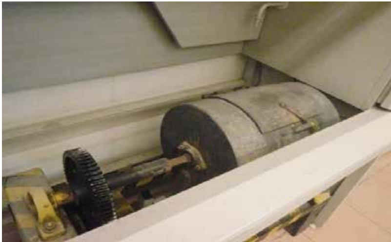
Fig. 7. The furnace used for heating the shredded particles to form a paste
