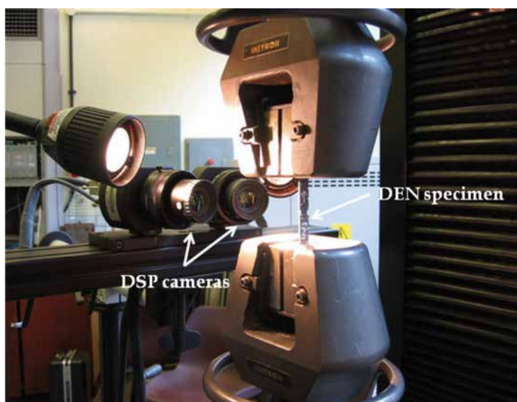
Fig. 9. Experimental setup for DEN specimens
