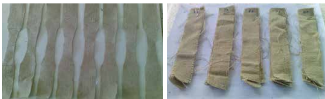
(a) Ramie woven for tensile testing
