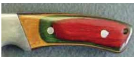
Fig. 22. Colored knife handles from veneers with MMA monomer and dyes
