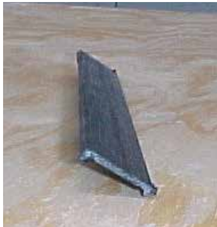
Fig. 19. U-Shape GF/PP pultruded profile made from towpregs
