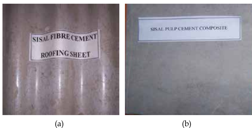
Fig. 7.3.1 Sisal composites: (a) Sisal fiber cement roofing sheet (b) Sisal pulp cement composites panel
