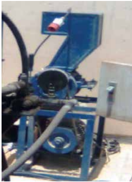
Fig. 6. The shredder adopted in crushing the extrudates
