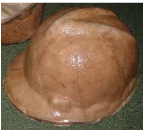
Fig. 11. Preliminary design safety helmet ramie-garut biocomposite
