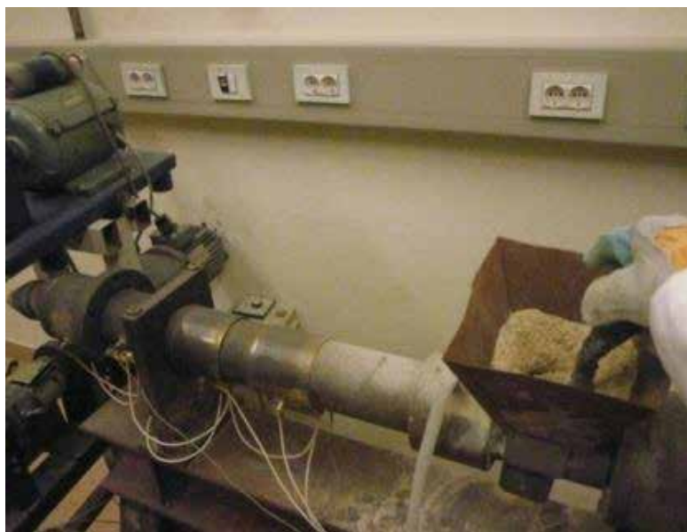
Fig. 3. Feeding the extruder with the mixture
