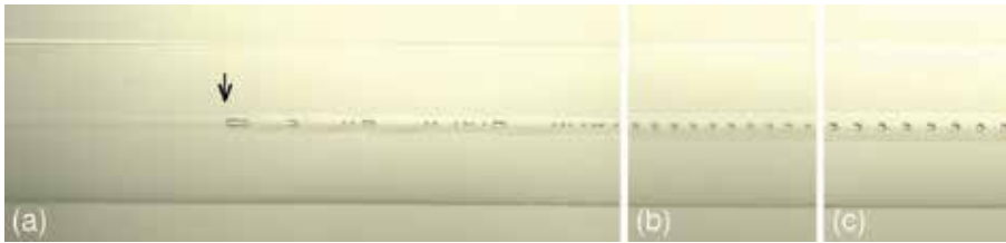
Fig. 6. Fiber fuse damage train in a standard single mode fiber (Corning SMF-28). After the ignition of the fiber fuse, the pump power of the laser ( 1.48 \mu\text{m} ) decreased from 7 W (c), 3.5 W (b) to \sim 1.2 W (a) until its self-extinction at the position shown by the arrow.
