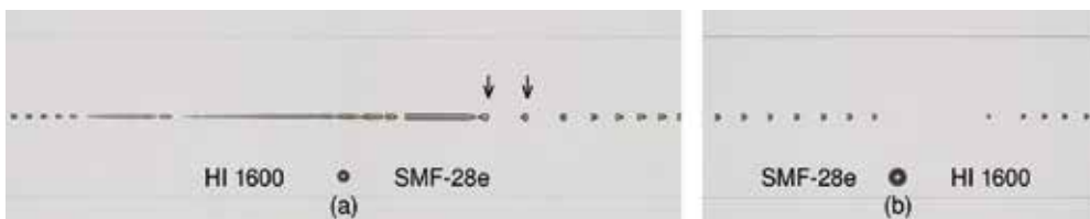
Fig. 21. Photographs of fiber fuse damage over the splicing point between HI 1060 and SMF-28e (Corning). The hollow spheres in the cladding are located at the border between two fibers and were accidentally captured during splicing. The fuse was initiated with 9W 1.07\ \mu\text{m} light that propagates in a multi-mode through SMF-28e.
