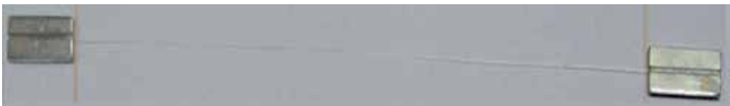
Fig. 1. Photography of a tested optical fiber with the glued aluminum plates on the extremities.
