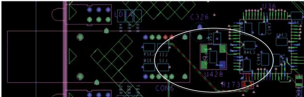
Fig. 16. Unrouted differential lines.
