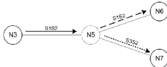
Fig. 5. Example Link-by-Link routing, Unicast S_1 : \{N_3\} \rightarrow \{N_6\} , Multicast S_2 : \{N_3\} \rightarrow \{N_6, N_7\} , and Unicast S_3 : \{N_5\} \rightarrow \{N_7\}
