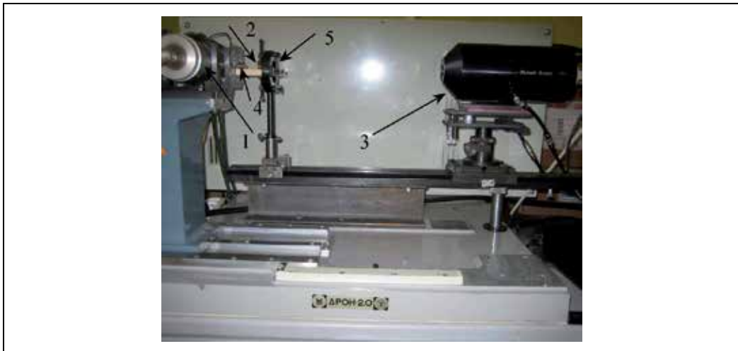
Fig. 11. X-ray microscope. 1- X-ray tube; 2- X-ray lens in a holder; 3- CCD X-ray camera; 4 - object for imaging; 5- goniometer for X-ray lens.
