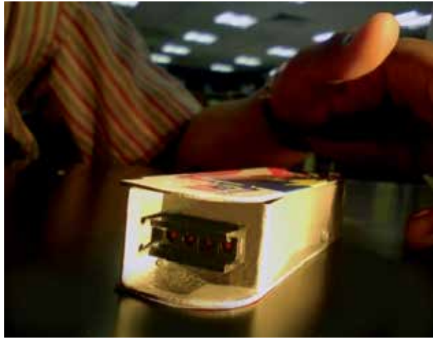
Fig. 9. Prototype of 1 \times N GT-POF splitter. The input signal is split into four channels which are suitable to distribute the application equally to the number of destination
