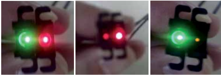
Fig. 10. Prototype of the 1 \times N POF Demultiplexer. The device is used to split the signal to different frequency (color). The multiplexed signal is separated according to the application (data & video signal) respectively
