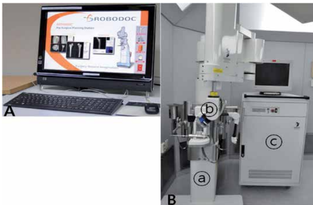
Fig. 9. ROBODOC® system (Integrated Surgical Systems, Davis, CA) is composed of two primary components. (A) CT-based preoperative planning using ORTHODOC, and (B) Robot-assisted surgery using the ROBODOC surgical assistant (Ⓐ = robot base, Ⓑ = robot arm, Ⓒ = the control computer)
