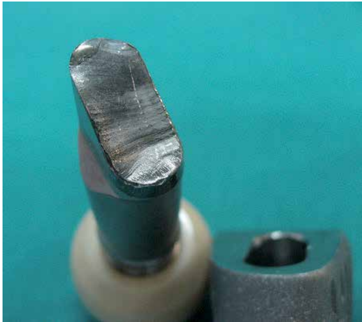
Fig. 3. A close-up photograph showing the fractured modular femoral neck.
