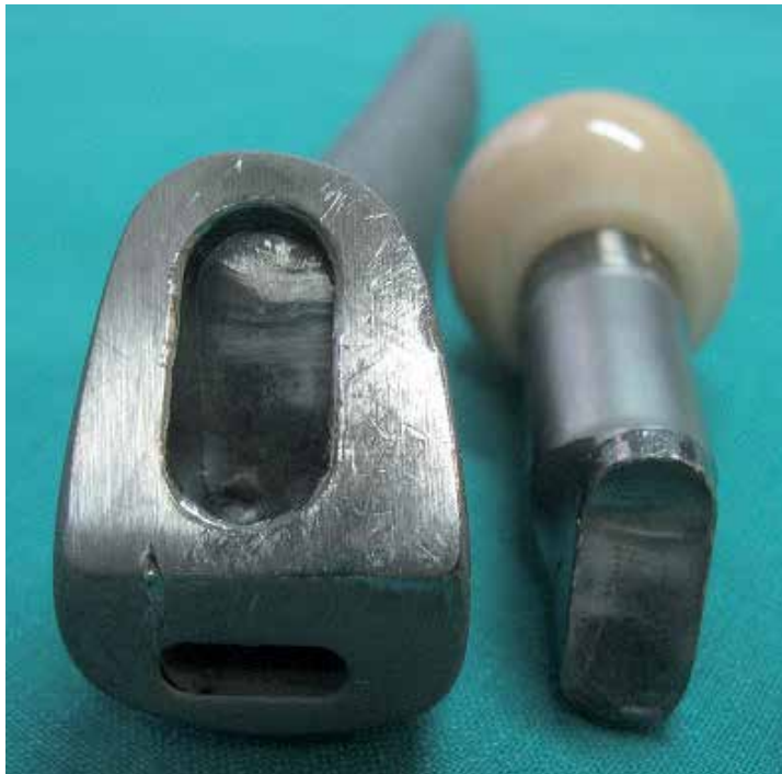
Fig. 4. Photograph showing the removed prosthesis with fractured neck and the remaining of the modular neck in the femoral stem taper.
