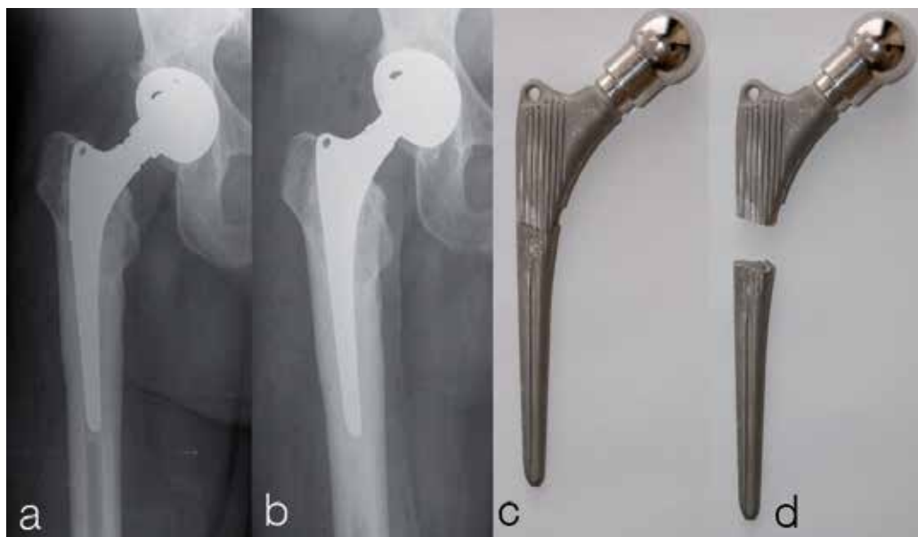
Fig. 3. a: Femoral component failure 14 years following primary surgery. b: Revision with normal femoral component following retrograde removal of broken stem. c and d: Removed, broken component.
