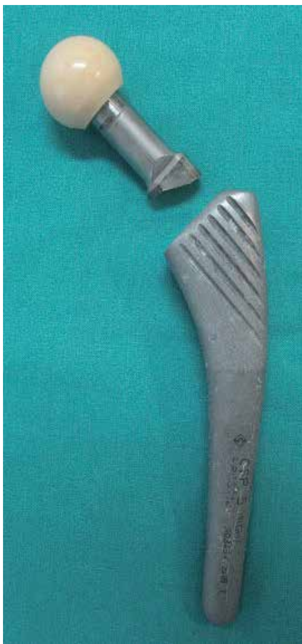
Fig. 2. Photograph of the retrieved fully-modular prosthesis showing the modular neck fracture.
