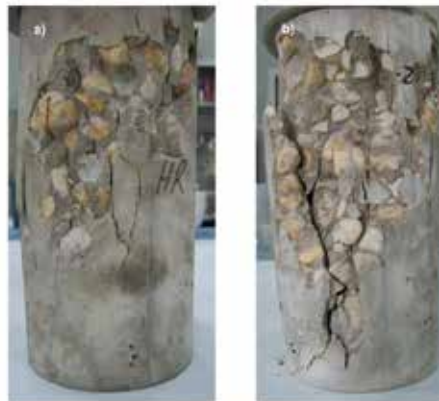
Fig. 3. Types of compressive fracture: a) Concrete CC. b) Recycled concrete RC-25
