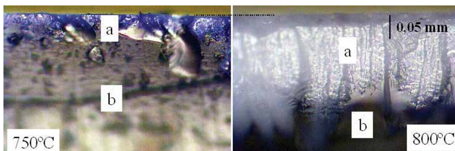
Fig. 4.17. Optical photographs of the cross section of the 60SiNa samples surface treated at 750 and 800 °C (a - crystalline zone (film), b - glass matrix). 20x magnification.
