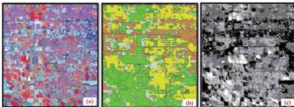
Fig. 5. (a) Landsat color infrared image of T3NR1E of the Boise Valley; (b) Land use/land cover polygons in T3NR1E of the Boise Valley; (c) ET image of T3NR1E the Boise Valley (after R.G. Allen et al., 2007)
