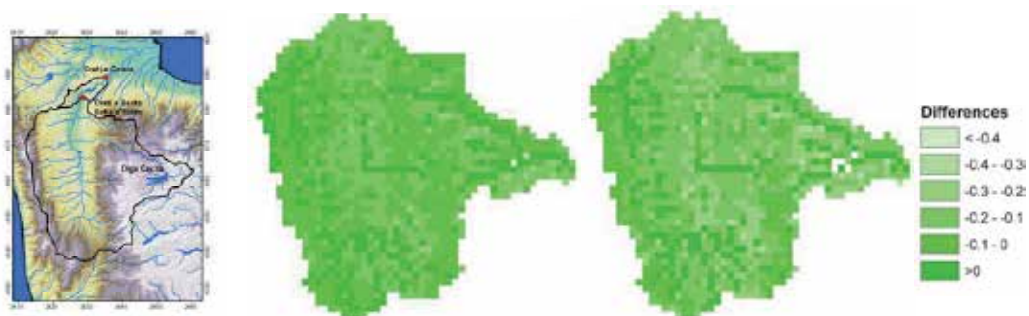
Fig. 15. Location of the Crati River Basin (left) and spatially distributed percentage changes in annual actual evapotranspiration (middle) and in actual evapotranspiration during the April-September irrigation period (right) simulated using RegCM (2070-2099 vs 1961-1990) (adapted from Senatore et al., 2011).
