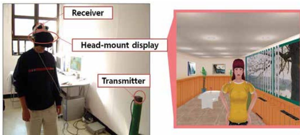
Fig. 2. Virtual reality social encounter task for measuring personal space. A participant is wearing a head-mounted display and enters into a virtual room. A receiver is placed on the vertex of the participant and represents the position and head orientation from a transmitter. A computer system calculates the distance and angle of head orientation from an avatar on the basis of the information from the receiver.
