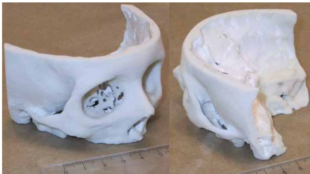
Fig. 8. Real 3D model produced with Rapid Prototyping technique
