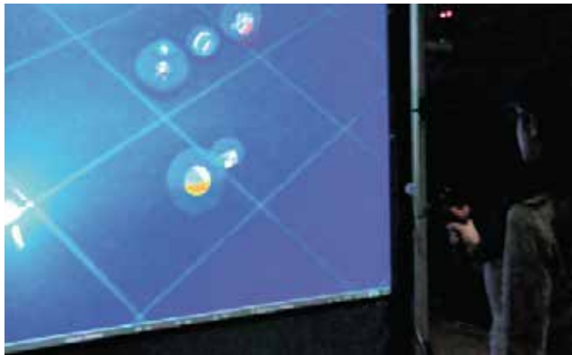
Fig. 12. The EVR@ platform with a user using a Flystick to interact in the virtual environment.
