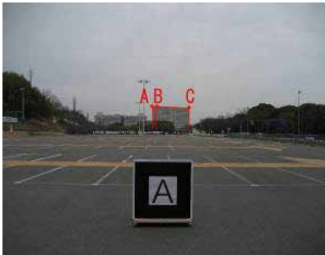
Fig. 14. The marker, actual building, and virtual 3D CG object. Distance between the marker and the building = 964m.
