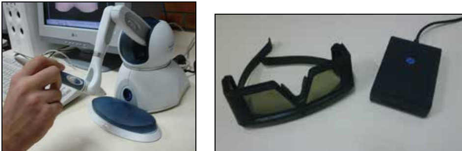
Fig. 5. 6DOF haptic device (left) and shutter glasses for stereoscopic visualization (right).
