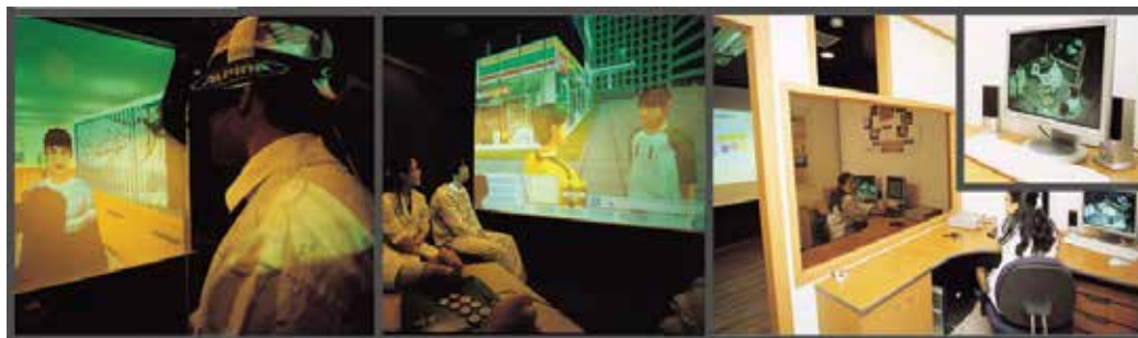
Fig. 1. Virtual reality presentation chamber. The chamber consists of the meeting room and the monitoring room. The meeting room is equipped with a head mounted display, a tracker, a beam projector, a screen, a camcorder, a speaker, and so on. In the monitoring room, a computer system controls all facilities in the meeting room and a situation in the meeting room can be observed through a one-way mirror.
