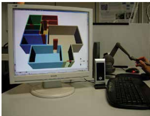
Fig. 2. The hapto-acoustic version of the World in Miniature metaphor used to navigate VE. The user pilots the avatar through the haptic stylus of a PHANToM Desktop
