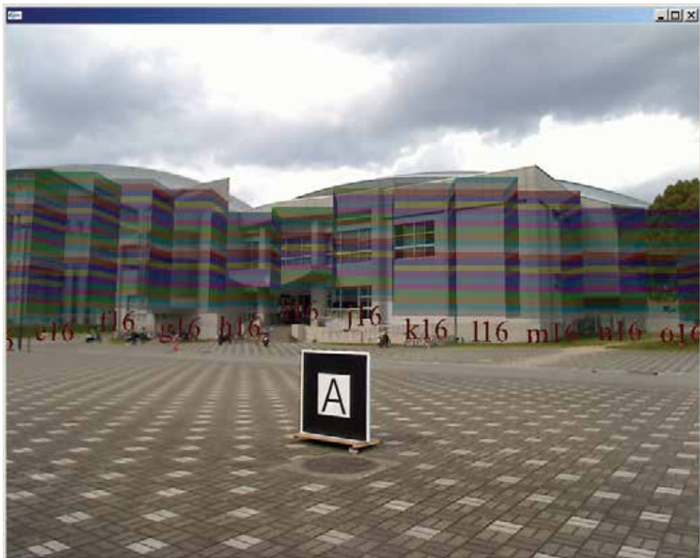
Fig. 12. A screen shot of the video image of the real buildings and marker with 3D CG scales of the 16th row, of which height are shortened so that they comply with the proposed regulation plan
