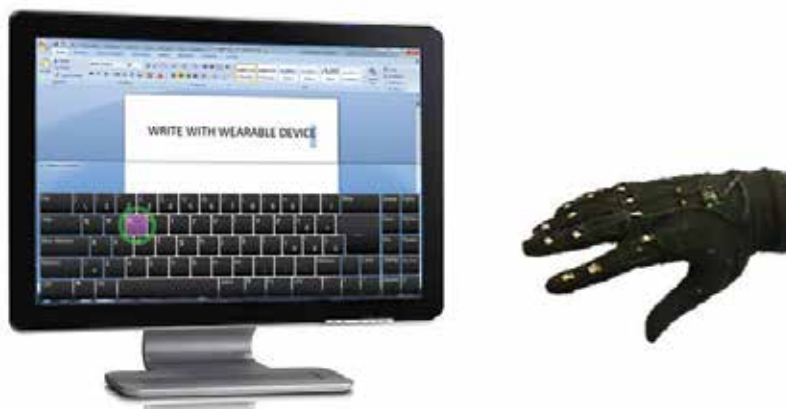
Fig. 4. Mouse and keyboard are unnecessary if computer interactions are made by a sensorized glove capable to accept commands obtained by finger motions.
