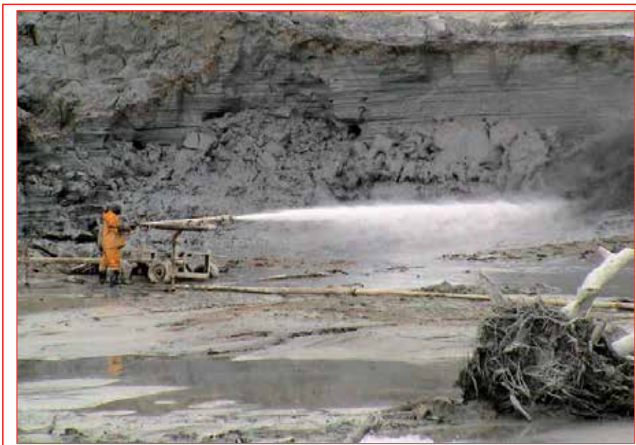
Fig. 2. Monitoring method being used for preparing slimes tailings for reprocessing at Crown Mines.
