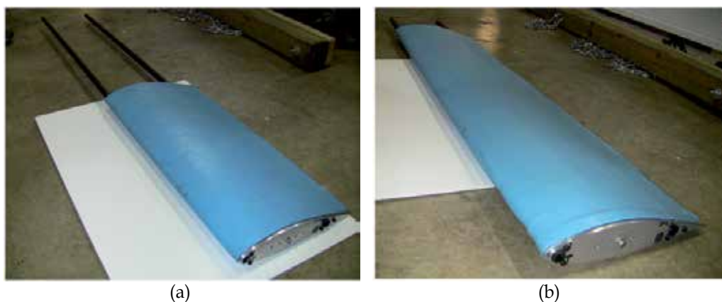
Fig. 21. Prototype morphing wing demonstration – (a) resting length, 0% morphing; (b) 61.0 cm span extension, 100% morphing.
