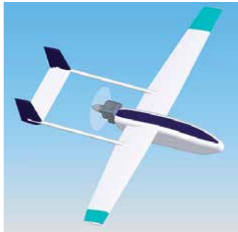
Fig. 1. Illustration of span-morphing UAV showing 1-D morphing wingtips.
