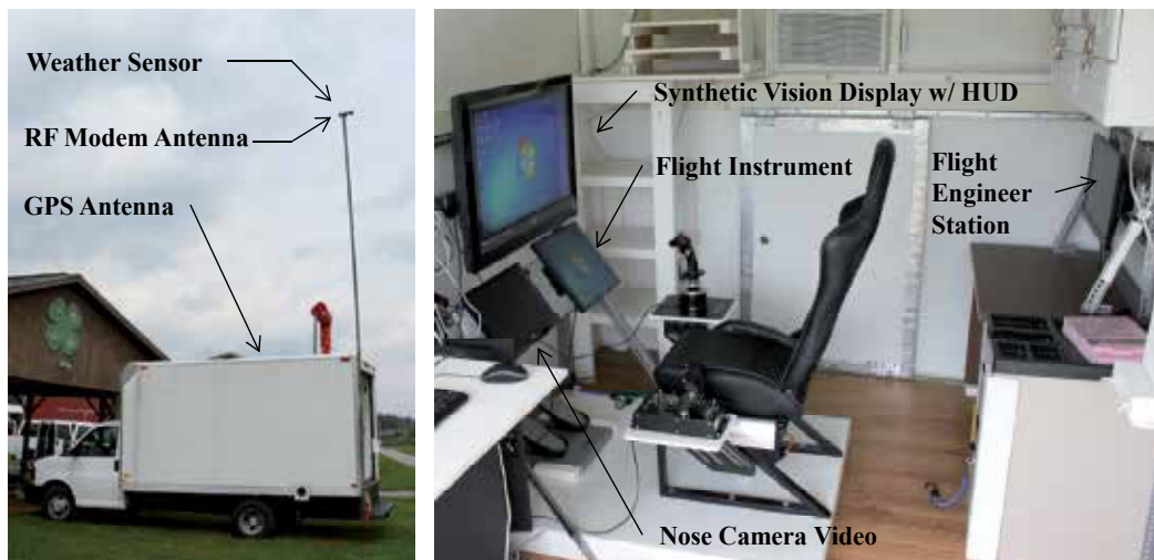
Fig. 4. The exterior (left) and interior (right) of the ground control station vehicle.
