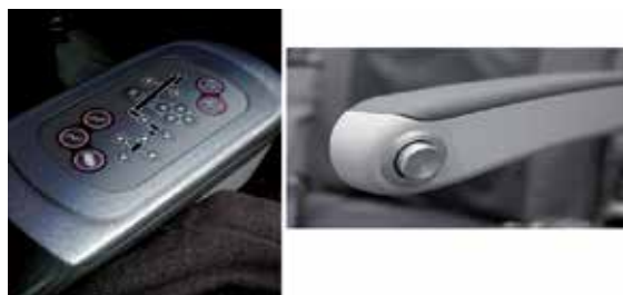
Fig. 3. Electronic Vs Mechanical seat adjustment
