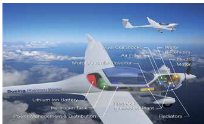
Fig. 33. Boeing PEM Fuel Cell Powered Electric Aircraft [36].
