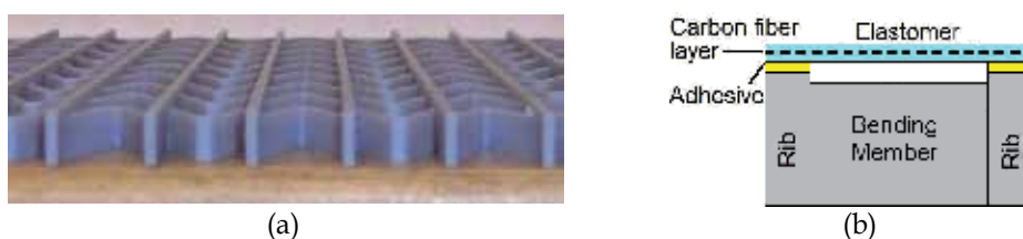
Fig. 13. EMC-structure bonding method – (a) honeycomb core; (b) single cell diagram.
