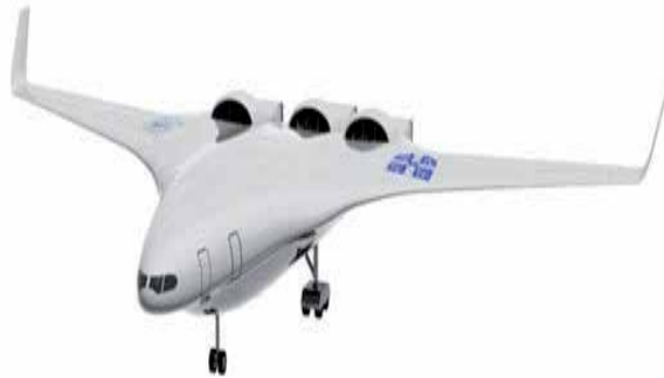
Fig. 12. Silent aircraft SAX – 40: (joint MIT/Cambridge University design) [12].
