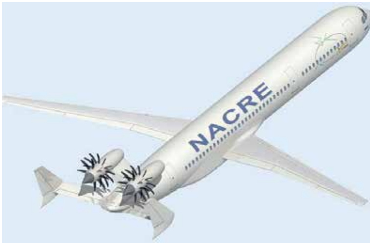
Fig. 21. Open-Rotor version of pro-active Green Aircraft in NACRE study [17].
