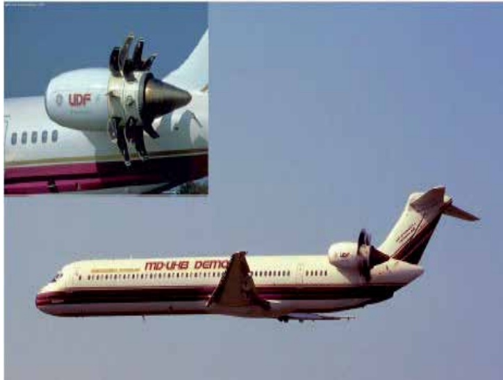
Fig. 20. GE36 Turbo-Prop demonstrator engine on MD-81 aircraft [21].
