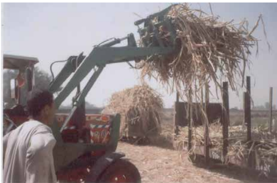
Fig. 13. Mechanical loading of light railway wagons using a tractor mounted loader (developed by the author).
