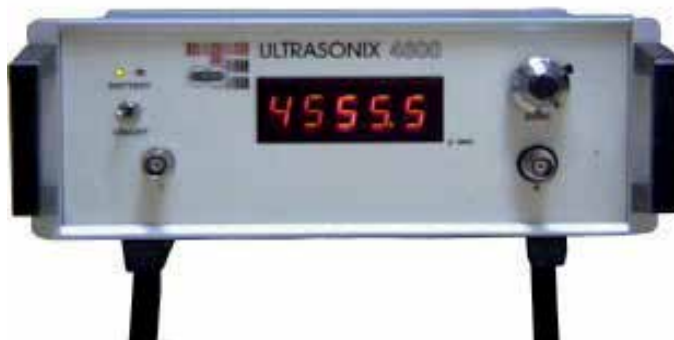
Fig. 6. Compressional wave velocity (P-wave) measuring device 'Ultrasonix 4600'
