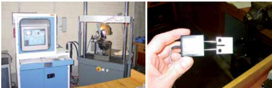
Fig. 9. Experimental tests for determining of J values
