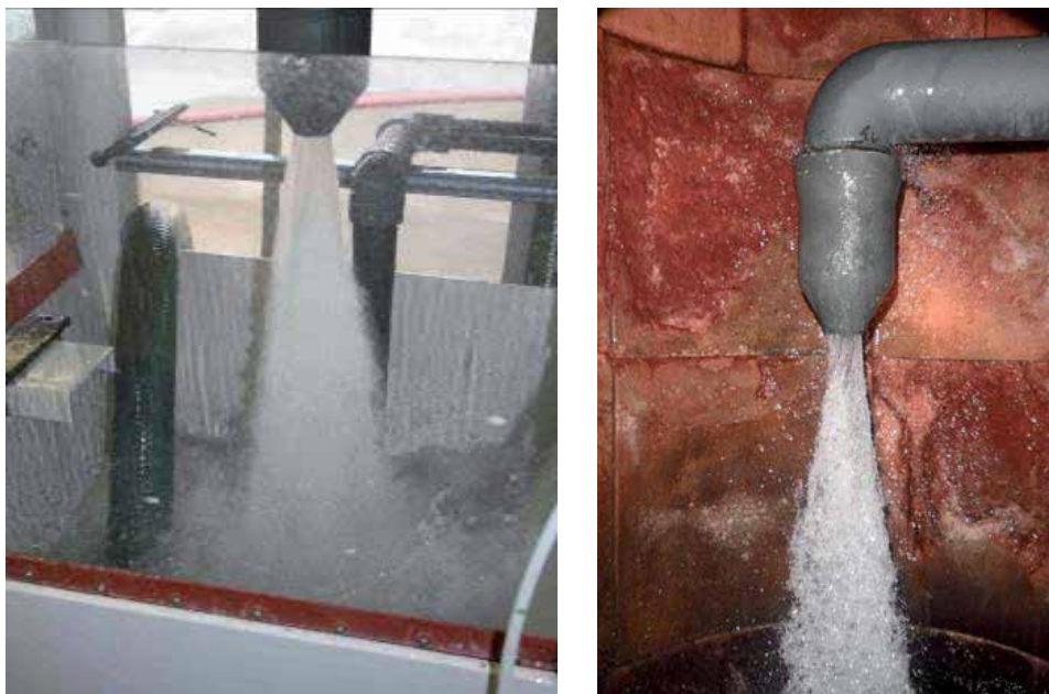
Fig. 2. Left, image of an axially-vaned thermal quench nozzle in operation in the authors' test stand. The aim of this test was to quantify the spray angle and asymmetries of the plant nozzle. Several flow rates and nozzle designs were tested. Right, field test in plant.
