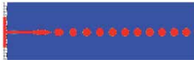
Fig. 14. Predicted droplets formed due to the Rayleigh-Taylor instability using the VOF method, showing good agreement with measured droplet sizes.
