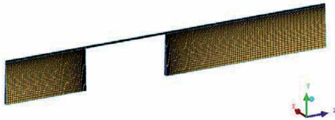
Fig. 11. CFD domain for the small sharp-edged cylindrical orifice case ( d=1 and l/d = 20 )
