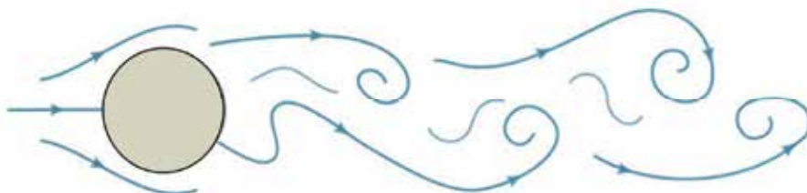
Fig. 1. The von Kármán vortex street observed in the wake region of a two-dimensional circular cylinder
