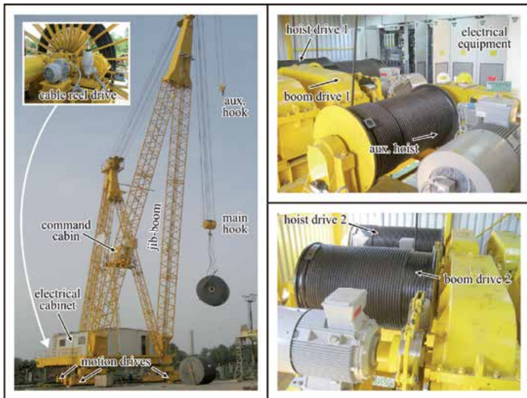
Fig. 13. Derrick crane with indicated drives.
