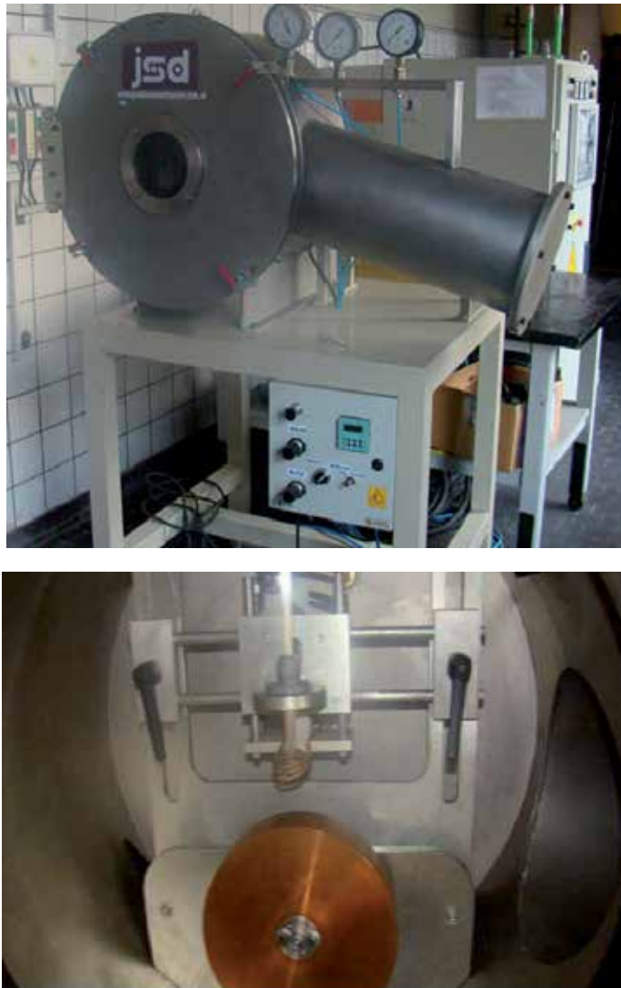
Fig. 4. Melt-spinning Equipment developed at LSA. Crucible and copper wheel.
