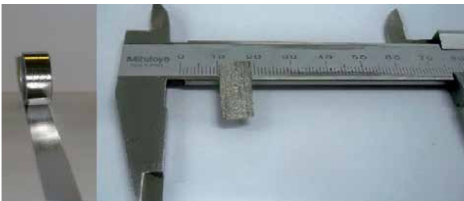
Fig. 13. Fe 78 Si 13 B 9 amorphous strips used in magnetic cores, and industrial magnetic package.
