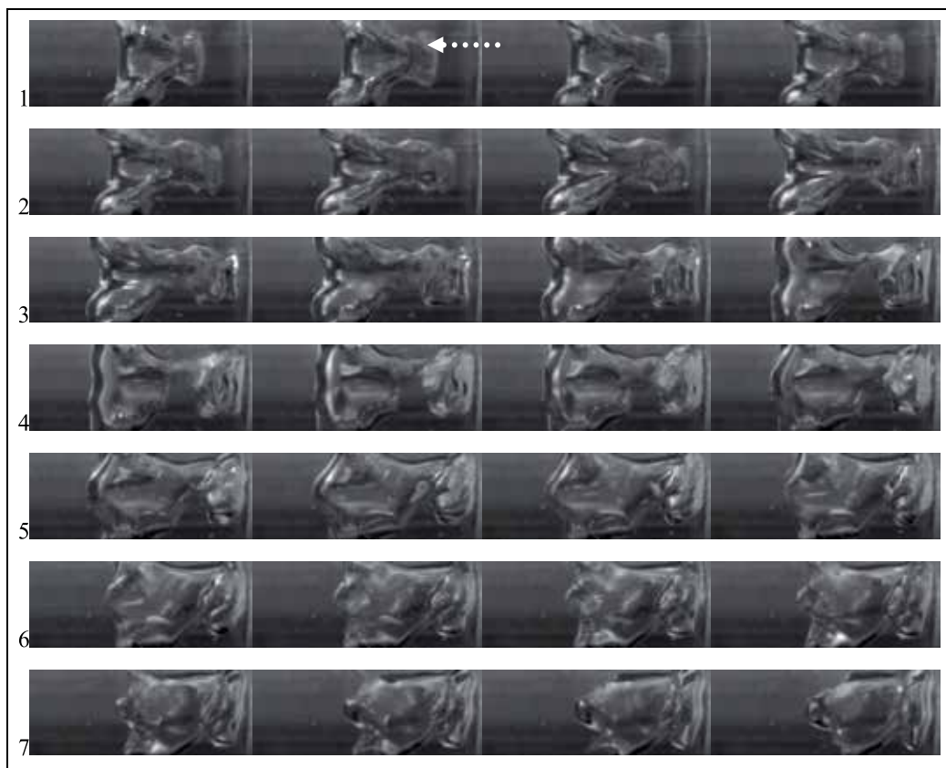
Fig. 10. Images of the process of bubble collapse at \gamma \approx 3 . The peak strength of the pressure wave is 300kPa. The size of each individual frame is 9.6 mm \times 3.1 mm. R_{\max} : 2.35 mm. The image time interval is 1/4000 second. (The Kelvin-Helmholtz vortex is indicated by a dotted line with an arrow).
