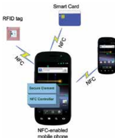
Fig. 4. NFC-enabled phone operating modes.
