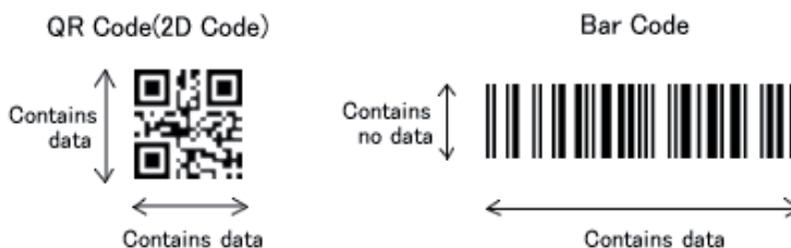
Fig. 2. QR Code compared with a Bar Code [Source: http://www.qrcode.com/aboutqr-e.html ]
