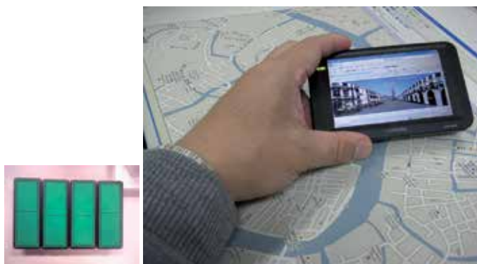
Fig. 3. Digital scope by a lightweight high-resolution display receiving data signal through the 2D sheet. The connector for the display contacts the sheet to receive the power signal.
