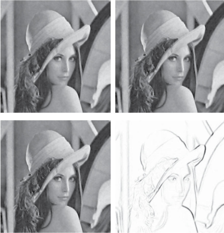
Fig. 4. Image restoration with the continuous TD algorithm R_{D_T} -Continuous (Aniso) for the Lena image with k_0 = 2 , upper row: \alpha = 0.10, 0.20 , lower row: \alpha = 0.30 and TD value for each pixel.
