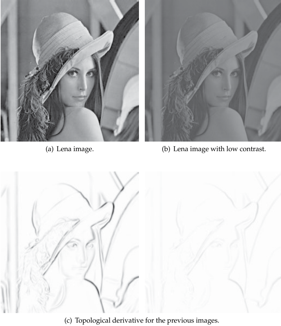
Fig. 5. Lena image with different contrast. The second row corresponds to the TD for each image using the same color scale in both cases.
