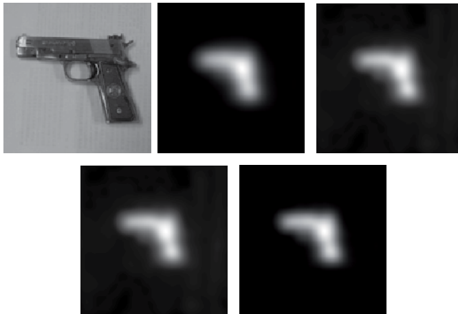
Fig. 17. (a) Visible Image (b) Captured Image (c) Standard Landweber (d) Projected Landweber (e) Adaptive Projected Landweber
