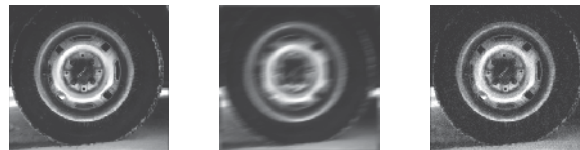
Fig. 9. Result for Tire . True image(left); blurred image (middle); restored image(right), BSNR=11.56, ISNR=22.09
