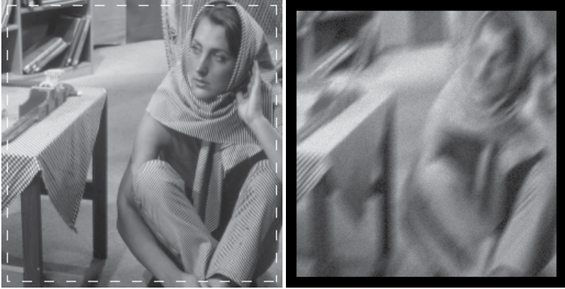
Fig. 6. Degraded and truncated image by diagonal motion blur (right) and the expected boundary region to be reconstructed (left).
