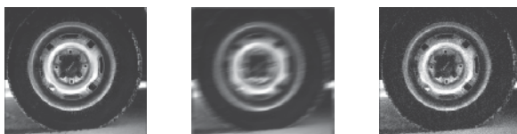
Fig. 5. RBFNN method result for Tire . True image(left); blurred image (middle); restored image(right), BSNR=11.22, ISNR=23.14
