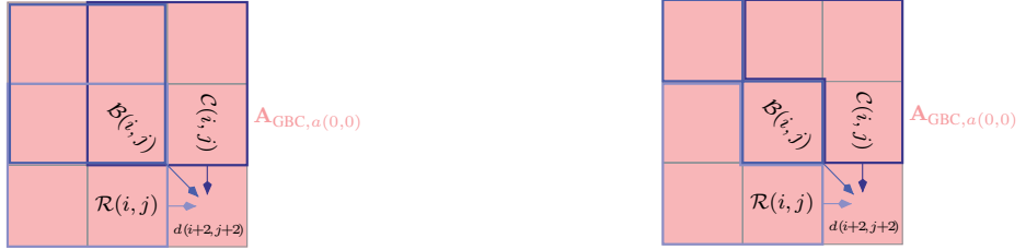
Fig. 14. The two possible layouts of auxiliary state variables \mathcal{R}(i, j) , \mathcal{C}(i, j) and \mathcal{B}(i, j) for the ISI channel \mathbf{A}_{\text{GBC},a(0,0)} .
